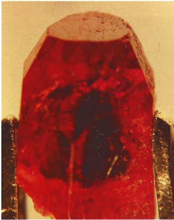
Figure 10. A well-formed Mong Hsu crystal consists of two hexagonal dipyrramids, \omega and n , the positive rhombohedron r , and the basal pinacoid c , as illustrated by this 5-mm sample. Note the violet core.
