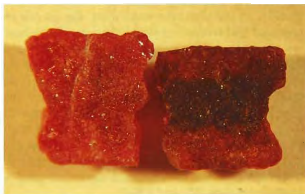
Figure 8. This 8-mm-long Mong Hsu crystal has been cut to show the effect of heat treatment on the core area. The right half is the original (untreated) control sample; with heat treatment, the left half is now a solid red.
