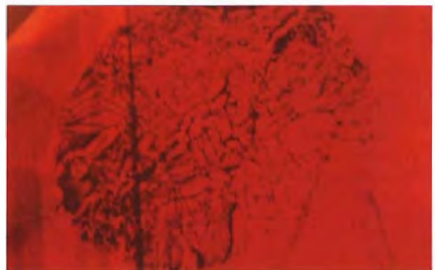
Figure 26. In some partly recrystallized fractures, it is difficult to locate the foreign substance (possibly borax or an aluminum borate) to which the ruby was exposed during heat treatment. Immersion, magnified 60x.
