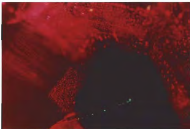
Figure 20. A whitish streamer (left) emerges from the end of a pseudosecondary feather of fluid inclusions along the black core of this untreated Mong Hsu. View almost parallel to the c-axis, fiber-optic illumination, transmitted and reflected light, magnified 60x; photomicrograph by E. Gübelin.
