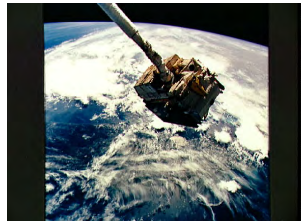
STS057-93-052 1993-07-01 EURECA is retrieved by RMS to be stowed in PLB for return to earth.
