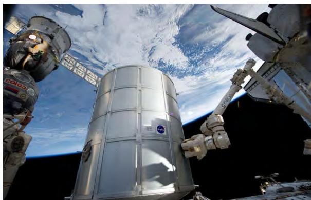
S133-E-007808 --- ISS's Canadarm2 grasps the Italian-built Permanent Multipurpose Module (PMM) for transfer from Discovery's payload bay to be permanently attached to the Unity node.
