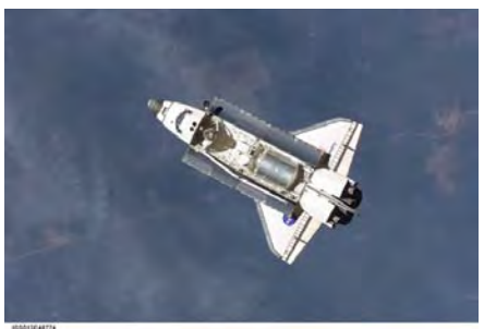
ISS013-E-48774 --- Discovery approaches ISS for docking with Leonardo Multipurpose Logistics Module (MPLM) in the payload bay.
