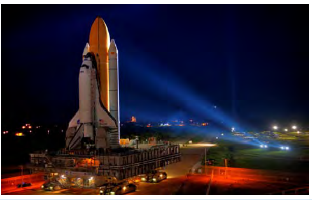
Giant Crawler Carries Shuttle To Pad ABOVE: STS-133 rolls to PAD on 09/20/10 for first launch attempt - scrubbed on 10/29/10. The KSC crawler-transporters (two) carried all Apollo Saturn V's and all Shuttle vehicles on the gravel path from the VAB to Launch Complex 39.
