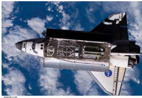
iss015e11705 S3 S4 PL: The 17.8 ton S3/S4 truss to be added to the station is shown berthed in the Shuttle payload bay.
