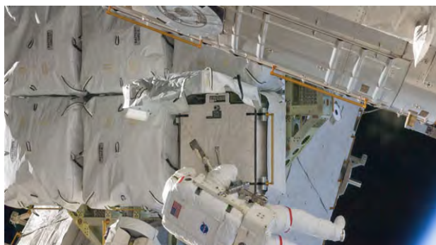
S132-E-008106 -- Bowen during first EVA with Reisman (out of frame), continues construction and maintenance on the ISS, with battery replacements & installation of a 2nd Ku-band antenna.
