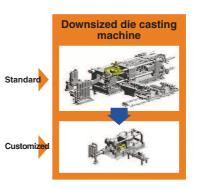
Improved die casting machine, developed by Toyota, is customized to reflect the shape of the finished product, costs 50% less than its predecessor, and has one-third the production lead time. (Source: TOYOTA Annual Report 2003)
