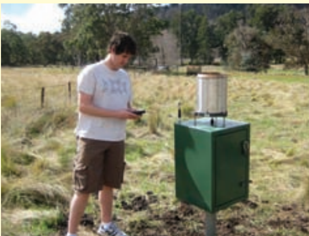
Testing the radio signal from an automatic rain-gauge at Nundle, near the head of the Peel River.
