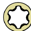
TORX Drive bit in TORX PLUS Drive fastener
