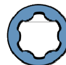
TORX PLUS Drive bit in TORX PLUS Drive fastener
