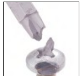
Concentrated stresses can cause breakage
