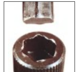
Tool and fastener damage is common
