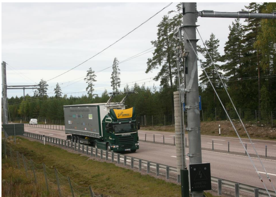
Figure 3-3: Conductive overhead ERS concept (©Maple Consulting, 2018)
