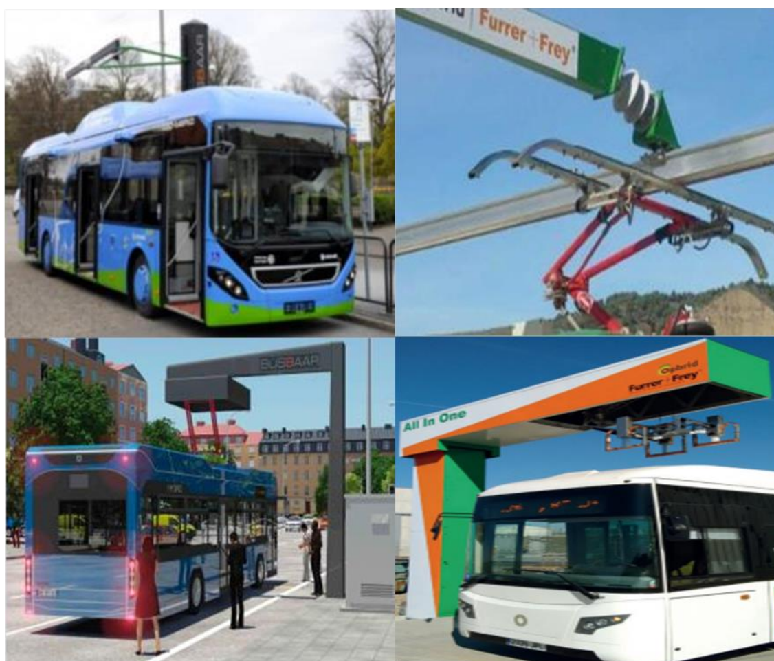
Figure B.16: F+F/Opbrid Systems (top left = V2 Busbaar,, top right = V2 pantograph, bottom left = V3 Busbaar, bottom right = All-in-One (Source: Furrer and Frey)
