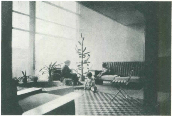
Fig. 14 LARGE WINDOW with diffusing curtain achieves excellent brightness distribution aided by reflected light from white walls and ceiling
