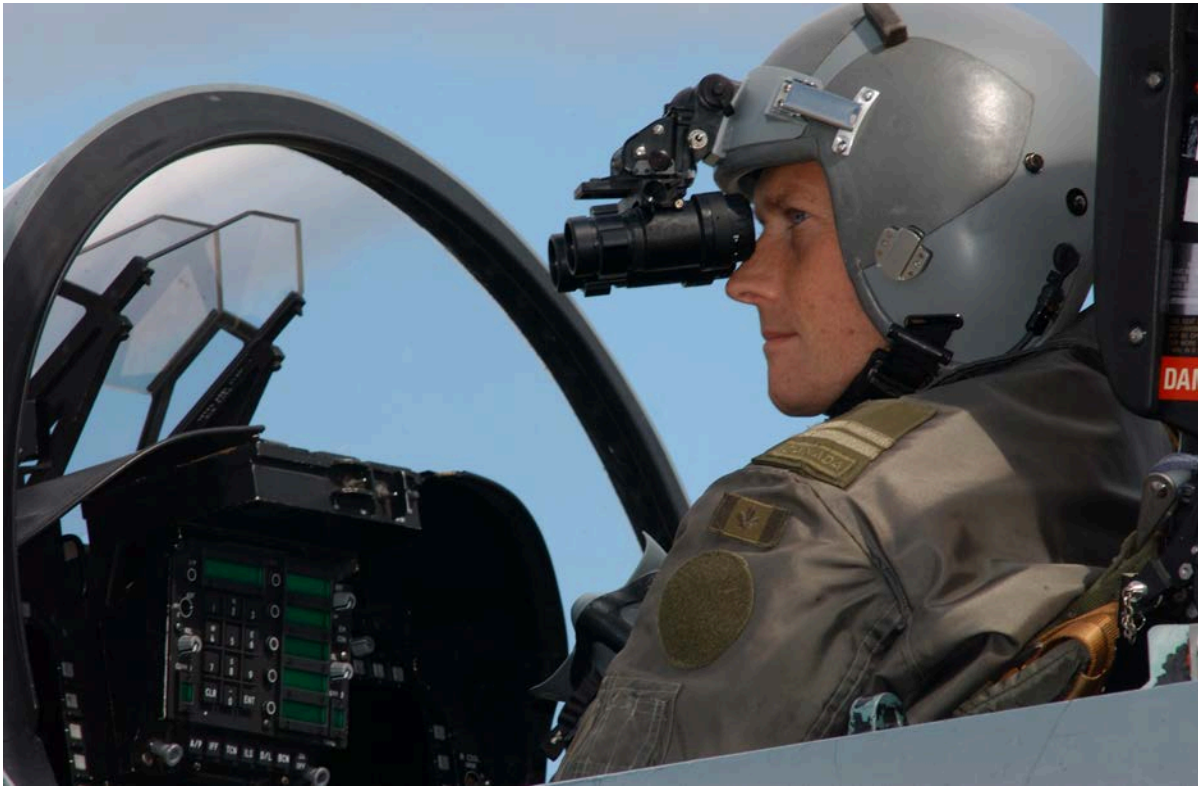
A pilot wearing night-vision goggles attached to his helmet - (CF Image - CX2005-0258-11d)
