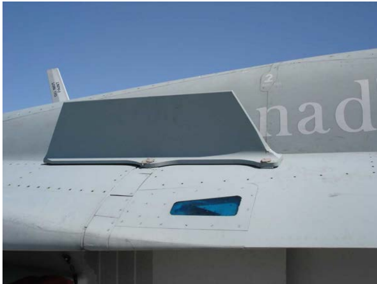
The aerodynamic fix for the vortex problem was the installation of this plate or "fence" on top of the fuselage - (CF Image)
