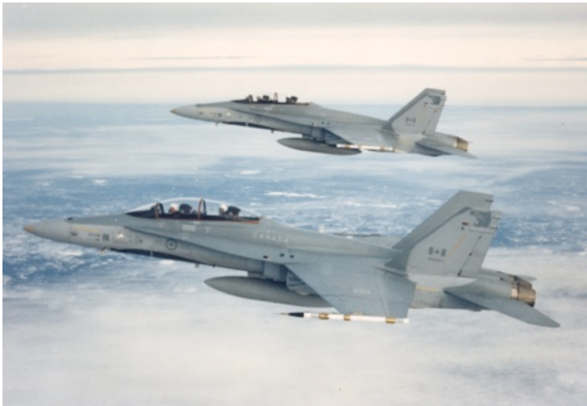
Below - CF188901 while in service with 410 Sqn carrying an AIS pod on the wing tip - (Bill Upton Collection)
