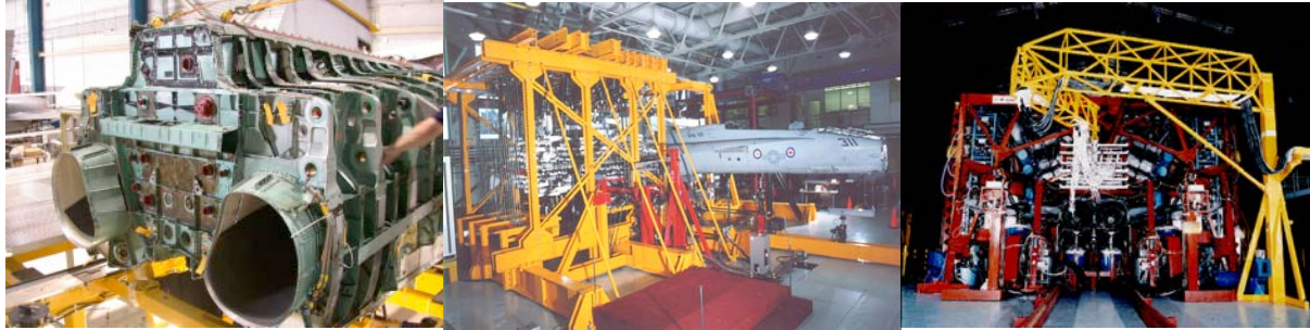
The complexity of the CF-18 structure and the IFOSTP testing is seen in these images. At the far left, the centre fuselage of the Hornet is revealed, the centre image shows the wing test underway at the NRC in Ottawa and the final image illustrates the aft-fuselage test in Australia - (NRC and ARML images)
