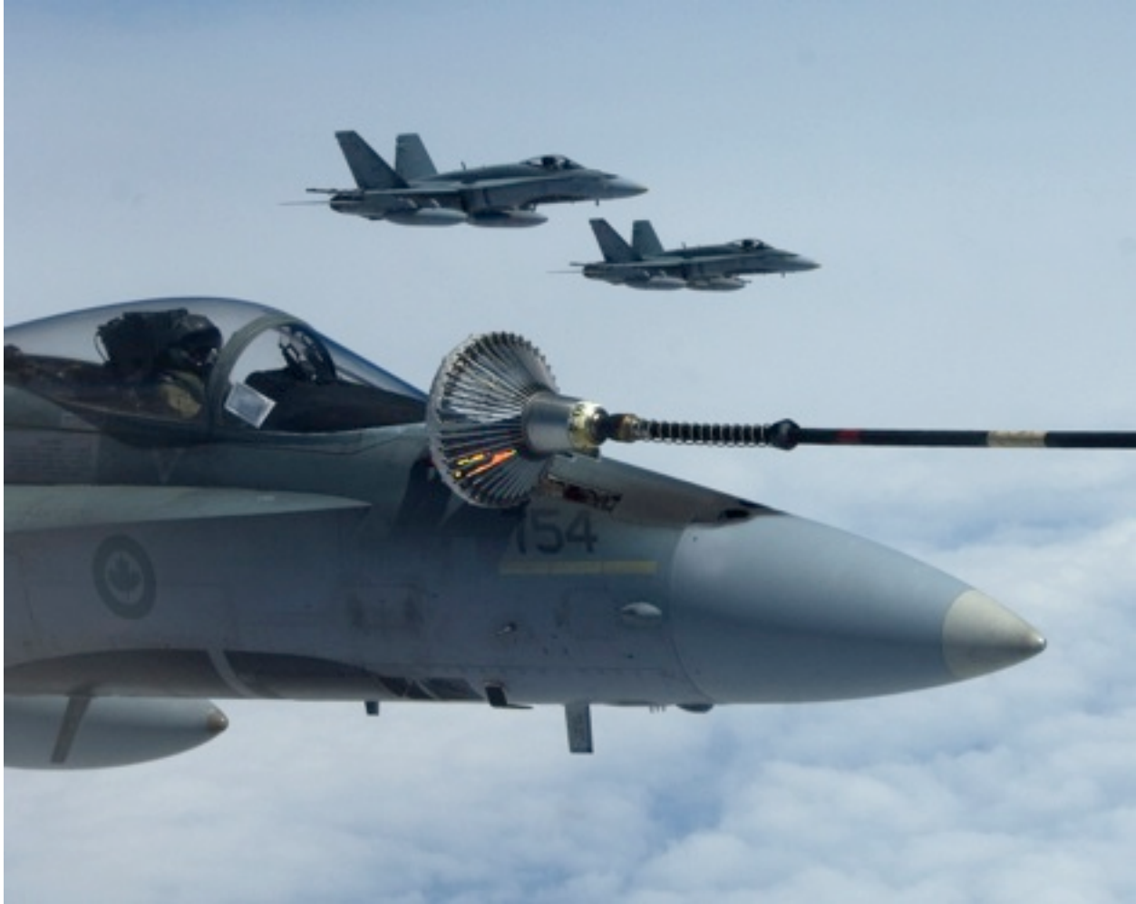
Above - CF188754 refueling using the probe and drogue system employed by the CC-150 tankers.
