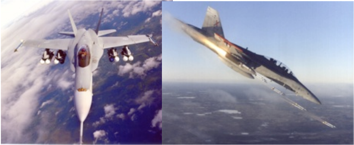
ABOVE - Two shots of CF-18 Hornets from the Aerospace Engineering Test Establishment (AETE) in Cold Lake performing weapon clearance tests. On the left, the aircraft is carrying eight BL-755 cluster bombs and on the right the aircraft is firing a LAU-5003 rocket pod containing 19 CRV-7 70 mm (2.75 in) unguided rockets. BELOW - A close-up of the installation LAU-5003 rocket pods on twin-store carriers for each of the underwing pylons. The CRV-7 rockets were fired through the frangible aerodynamic nose cones on the pods; an AETE CF-18 aircraft carrying the noticeably larger 2,182 litre (480 gallon) underwing fuel tanks; an AETE aircraft carrying a LAU-5003 and an Airborne Instrumentation Subsystem (AIS) pod and a CF-18 carrying the maximum load of ten Mk 82 "dumb" bombs equipped with high-drag tail fins - (CF Images & Bill Upton)
