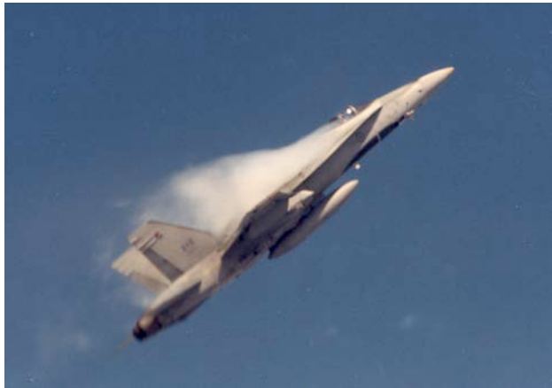
The vortices over the LEX are clearly seen here - (CF image)
