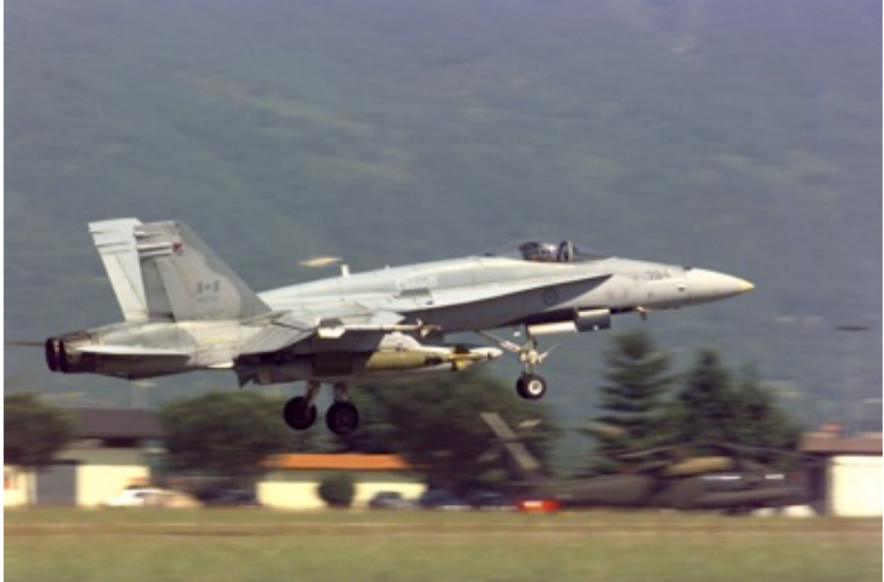
CF188794 lifting off for a mission over Kosovo. It is carrying a laser-guided bomb on the outer wing station - (CF Image - ckd99-2085-09)
