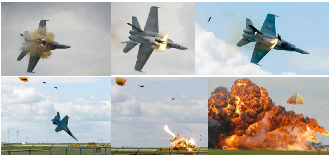
The effectiveness of the NACES seat is clearly demonstrated in this sequence from the crash of CF188738 in Lethbridge, Alberta on 22 July 2011. The pilot escaped with minor injuries after a low-level ejection - (CF Images)
