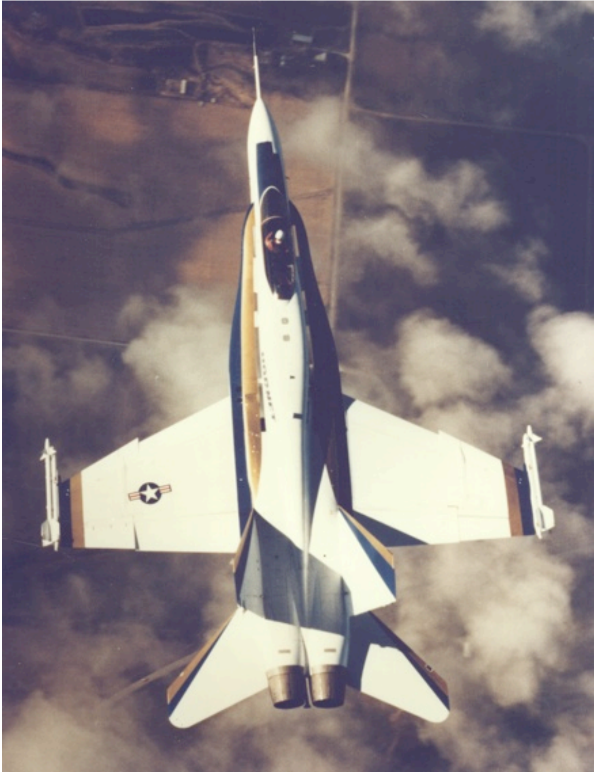
This overhead view of a prototype F/A-18 Hornet illustrates the trademark LEX extensions retained from the YF-17 design. Note also the slots in the LEX which later disappeared on production aircraft in order to solve aerodynamic issues - (Bill Upton Collection)
