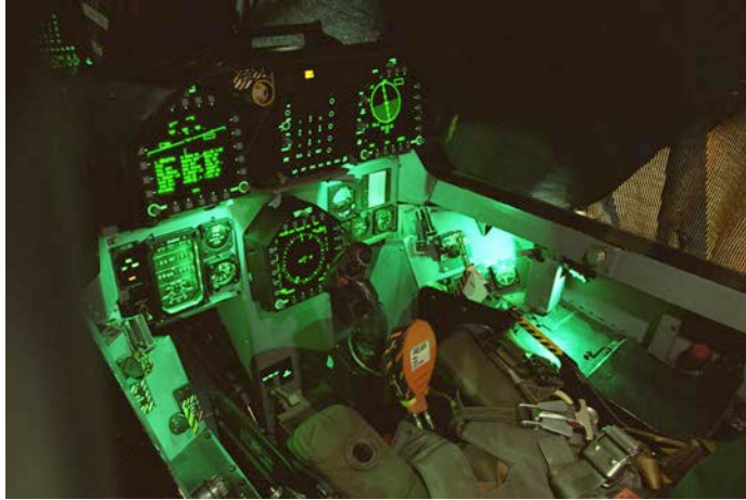
The new cockpit installation in the modernized CF-18 is fully night-vision compatible - (CF Image - CK00-0028-03)
