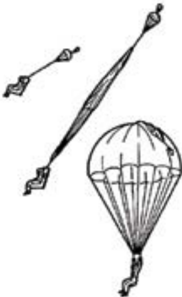
Figure 3a: SJU-9/10 Ejection Sequence - (CF Image)
