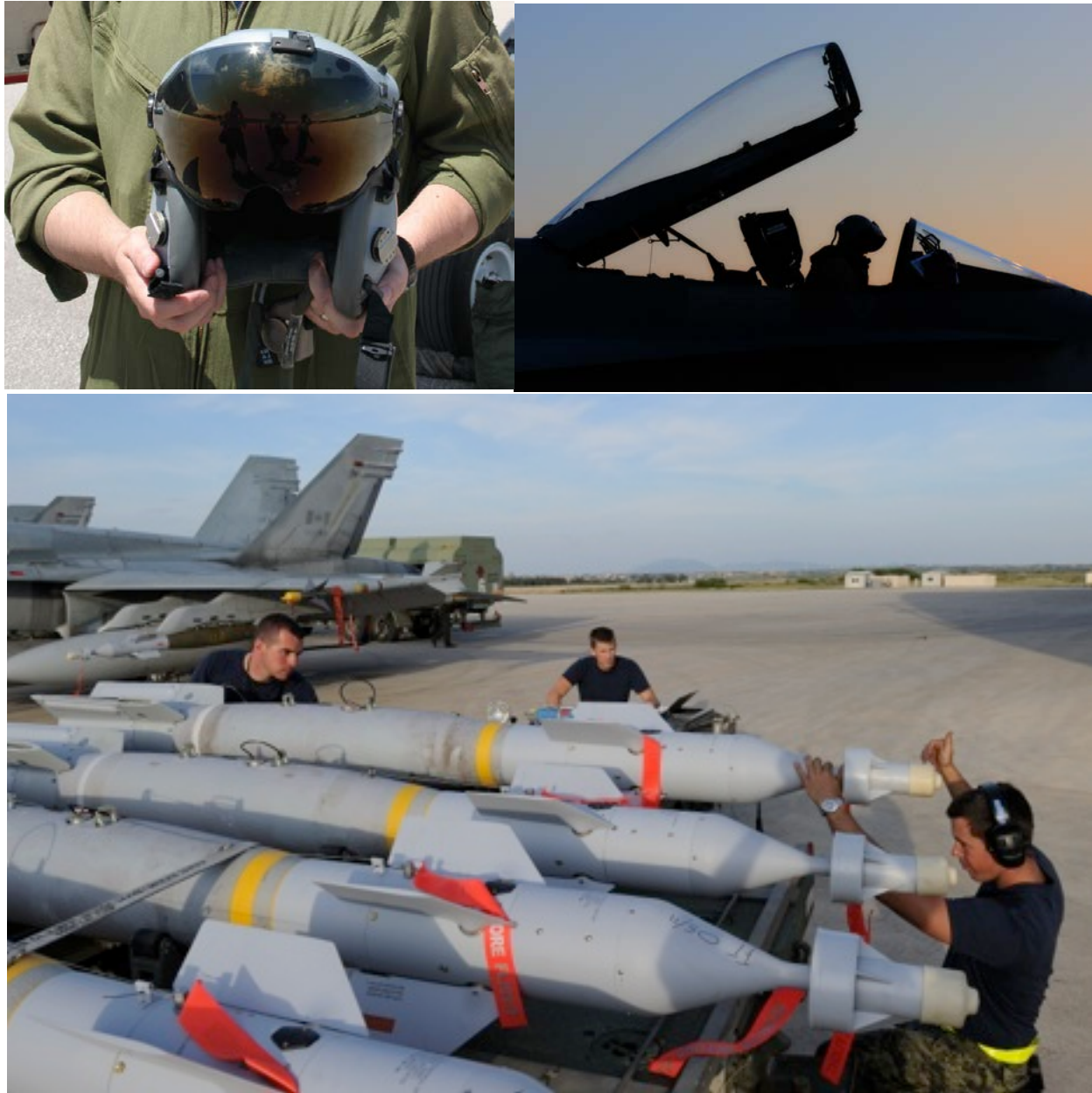
Top Left - the new JHMCS helmet provides information and visual cueing to the pilot on the helmet visor. Top right - a CF-18 pilot in the cockpit before a night mission in Libya. Bottom -RCAF armorers preparing laser-guided GBU-10 two-thousand pound bombs in Trapani, Italy - (CF Images - IS2011-4028-7, IS2011-M089-002, IS2011-4028-2)
