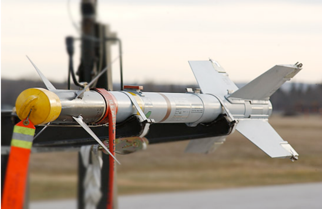
A close-up of the AIM-9 Sidewinder short-range missile. The AIM-9 is a heat-seeking air-to-air missile. Its heat-sensitive infrared (IR) guidance head enables it to home in on a target aircraft's engine exhaust - (CF image)
