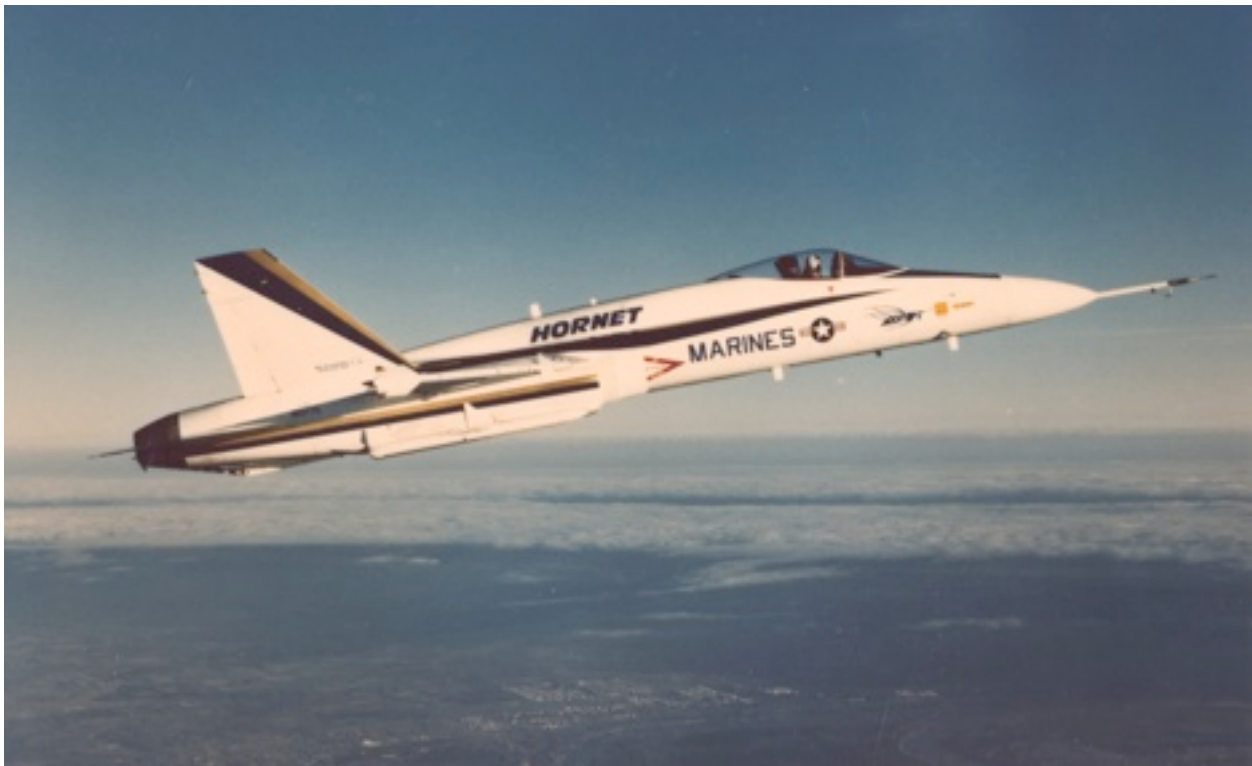
The prototype F/A-18 Hornet retained the basic planform of the YF-17 but not much else - (Bill Upton Collection)
