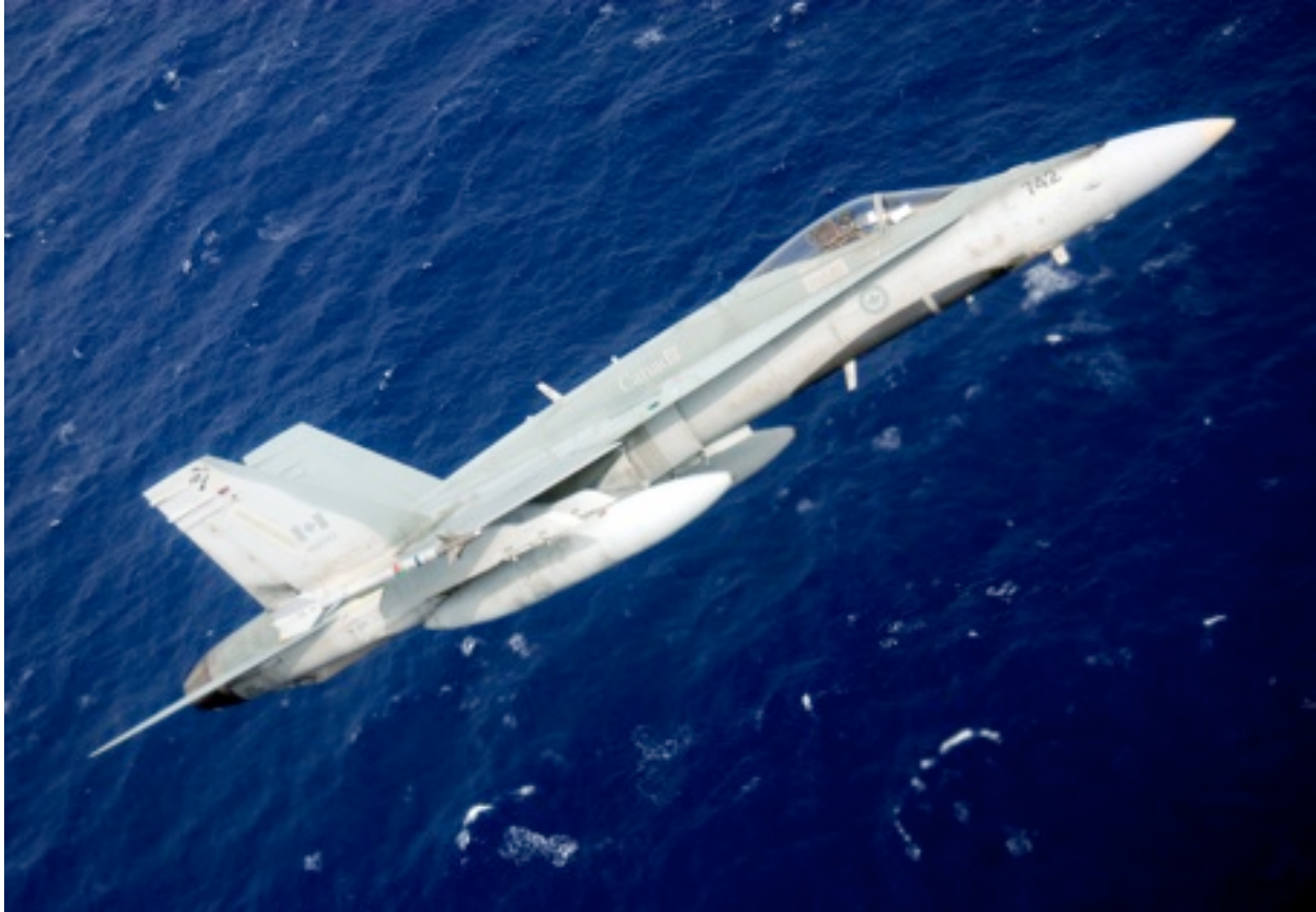
Externally the modernized CF-18 Hornet looks virtually identical to the older version. Extra blade antennas on the upper and lower fuselage and five IFF antennas on the nose of the aircraft are among the only visual clues. Internally, however, the aircraft is radically improved - (CF Image)
