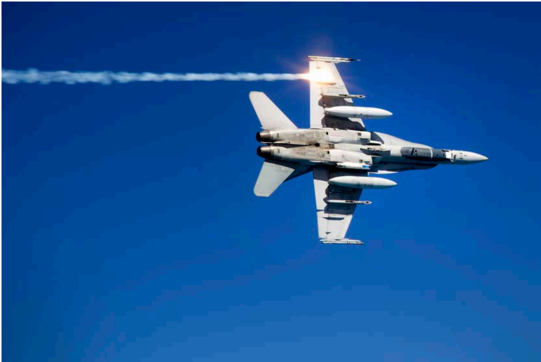
CF-18s also carry chaff and flare dispensers for self-protection. A flare, seen deployed here, would decoy incoming heat-seeking missiles away from the aircraft - (CF image)
