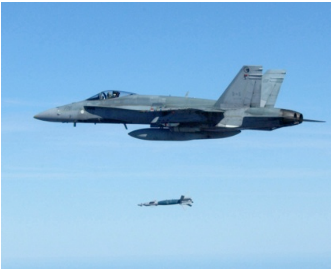
A CF-18 dropping a precision guided bomb. The weapon is steered to the target by reflected laser energy - (CF image)
