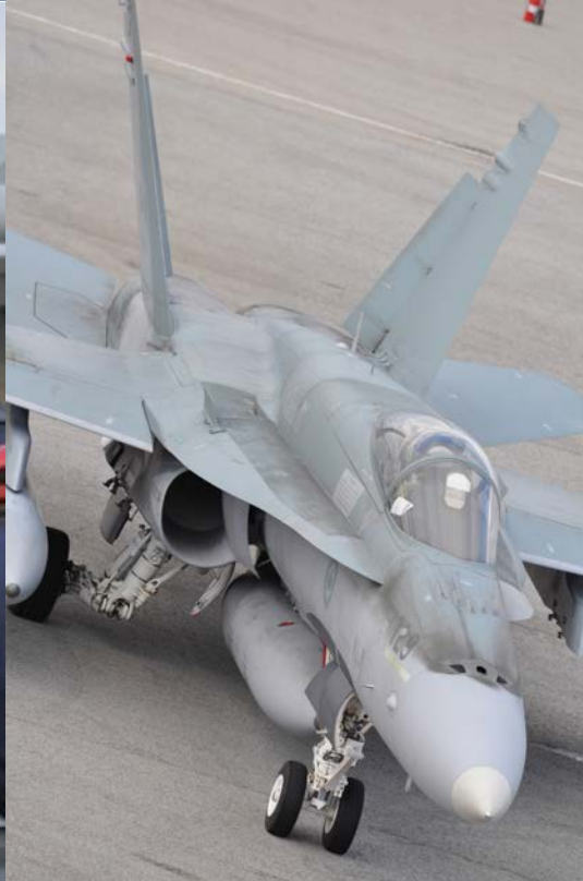
Top - In a scene reminiscent of a movie, a trio of CF-18s fire their AIM-7 Sparrow missiles, in this case against a practice target drone.. Lower left - the AIM-9 Sidewinder missile is typically carried on the outer wing launcher as shown here. Lower right - The CF-18 also carries a 20 mm cannon in the nose (the central hole in nose radome) with 578 rounds, with a firing rate of either 4,000 or 6,000 rounds per minute - (CF Images - Top - BN2011-0028-79)
