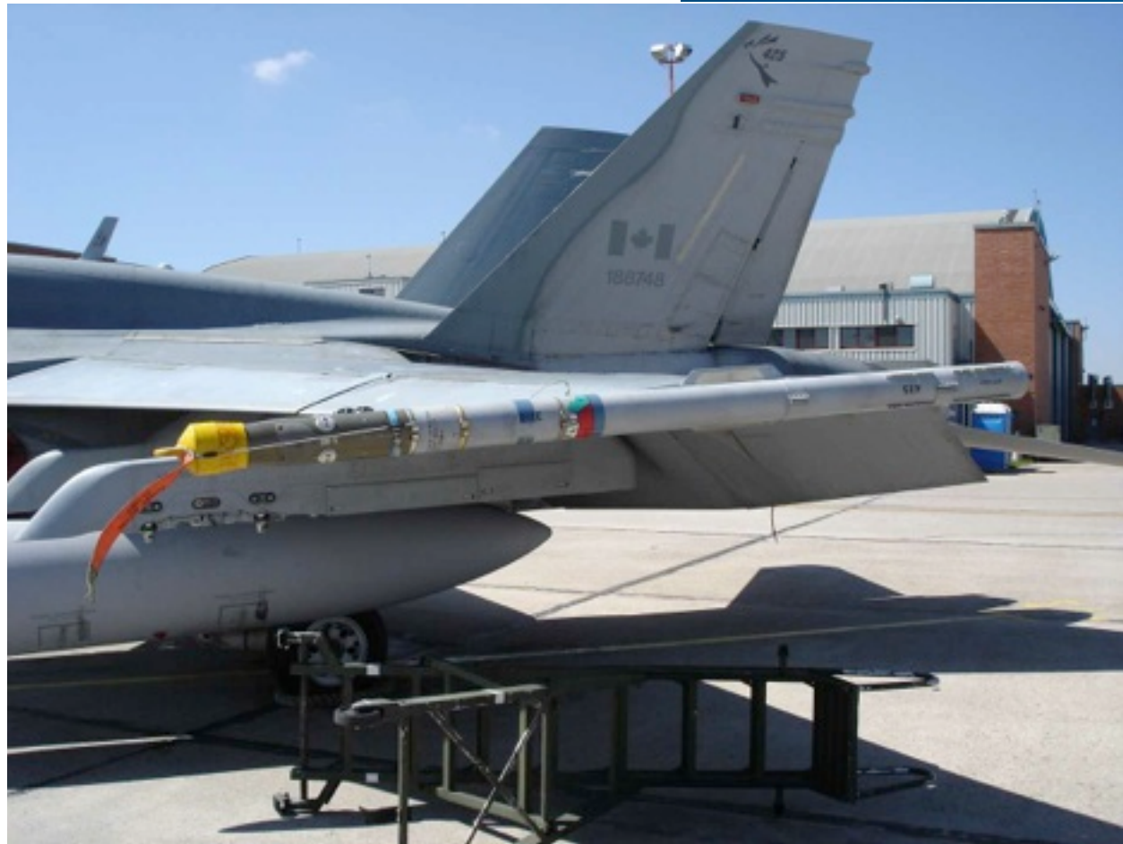
Clockwise from left to right - A close-up of the installation SUU-503 rocket pod and practice bomb dispenser on the outer wing pylon. An underneath view illustrates the SUU-503 from beneath. The false canopy design also shows up clearly in this same view. The Airborne Instrumentation SubSystem (AIS) Pod is carried on the outer LAU-7 launch rail in lieu of a missile. The AIS pod is used to provide real-time spatial positioning data for post-training mission debriefs - (CF images - AE2006-0039-016, AE2003-0053-003, & unknown # )
