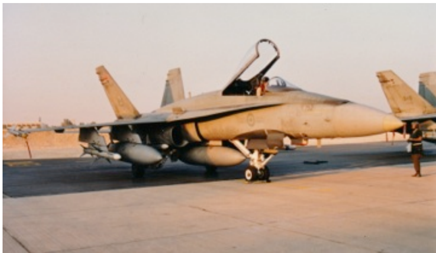
A Desert Cats CF-18 carrying an extra AIM-7 Sparrow on the outboard wing station - (CF Image)
