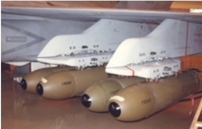
ABOVE - Two shots of CF-18 Hornets from the Aerospace Engineering Test Establishment (AETE) in Cold Lake performing weapon clearance tests. On the left, the aircraft is carrying eight BL-755 cluster bombs and on the right the aircraft is firing a LAU-5003 rocket pod containing 19 CRV-7 70 mm (2.75 in) unguided rockets. BELOW - A close-up of the installation LAU-5003 rocket pods on twin-store carriers for each of the underwing pylons. The CRV-7 rockets were fired through the frangible aerodynamic nose cones on the pods; an AETE CF-18 aircraft carrying the noticeably larger 2,182 litre (480 gallon) underwing fuel tanks; an AETE aircraft carrying a LAU-5003 and an Airborne Instrumentation Subsystem (AIS) pod and a CF-18 carrying the maximum load of ten Mk 82 "dumb" bombs equipped with high-drag tail fins - (CF Images & Bill Upton)
