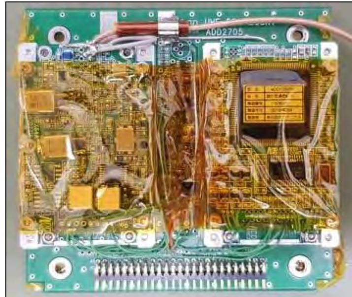
ADD2705. UHF transceiver board that has a heritage from BIRDS-3
