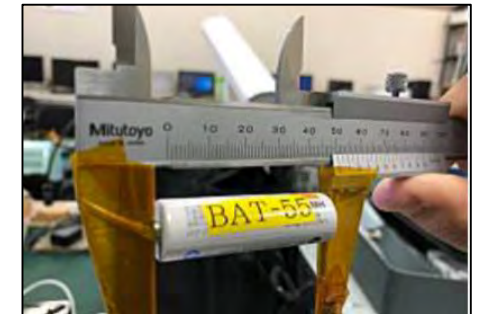
A scale and a caliper are used to measure battery weight and dimensions, respectively.
