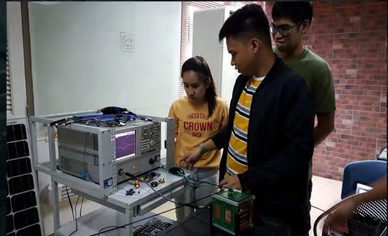
BIRDS 2S members checking the return loss plot of the VNA
