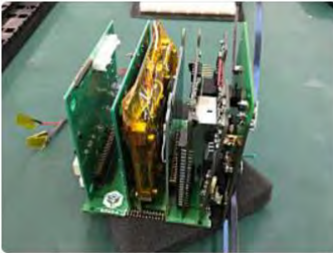
Integrated mission and subsystem boards without battery box
