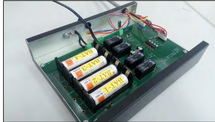
Battery charge-discharge hardware
