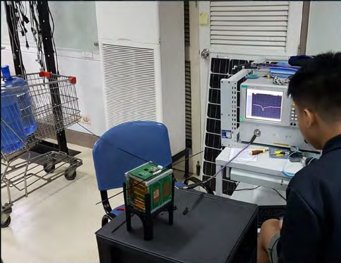
BIRDS 2S member Bryan Custodio tuning the antenna using VNA
