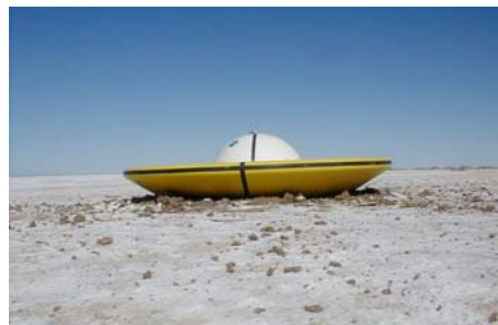
Figure 4: Full-size EEV Drop Model at UTTR
