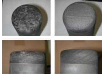
Figure 8: Carbon-phenolic after testing
