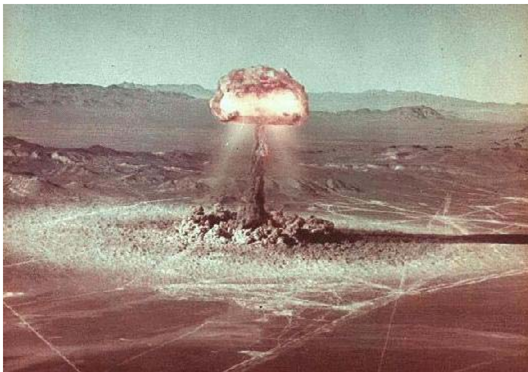
Fig. 11. The early stage mushroom cloud and stem several seconds after detonation. Note the shock effects on the surrounding ground and the formation of a base surge. From 'The Gallery of U. S. Nuclear Tests' web page: http://fas.org/nuke/hew/Usa/Tests/Busterj.html .
