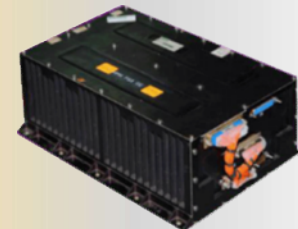
Actuator control electronics
