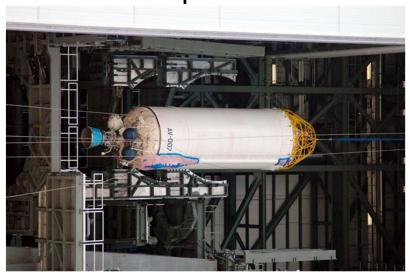
Centaur with a single RL-10A-4-2 engine Length 12.68 m Diameter 3.05 m Dry mass 2243 kg
