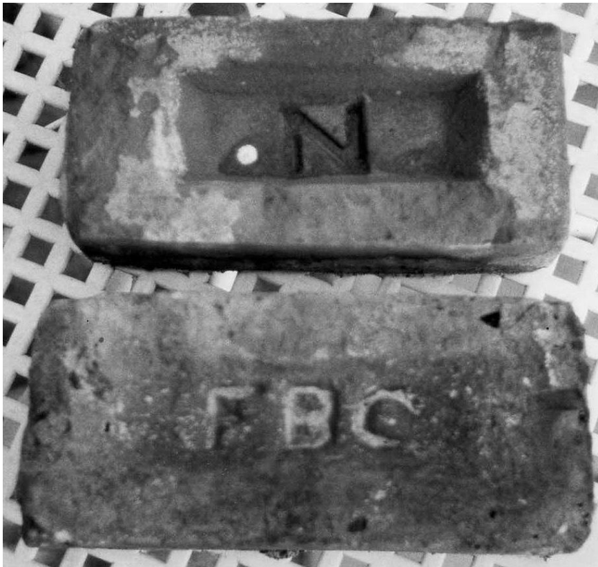
The same brick compared to a red brick from Newington Brickworks. It can be seen that the latter is slightly smaller and more uniform since it was not hand-made. The Newington Brickworks were owned by the same Ivory who was a partner of Frindsbury Brickfield before it closed.
