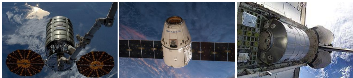
Figure 2. Cargo spacecraft. Left to right, the Orbital ATK Cygnus cargo spacecraft at the ISS, the SpaceX Dragon cargo spacecraft approaching the ISS, and the Space Shuttle delivering cargo to the ISS via the MPLM cargo carrier inside the Space Shuttle Discovery. Images NASA.
