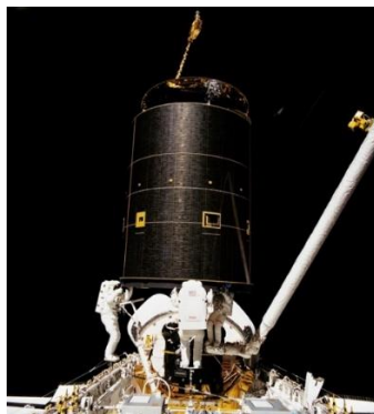
Figure 12. Space Shuttle STS-49 Endeavour Intelsat VI Repair. Astronauts Thuot, Hieb and Akers take manual hold of the satellite as commander Brandenstein delicately maneuvered the orbiter to within a few feet of the 4,215kg communications satellite. Image NASA.
