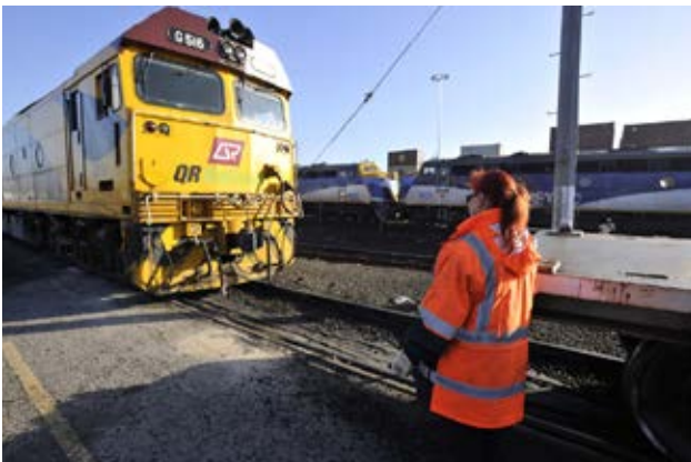
Shunters are the eyes of the driver who may be hundreds of metres away; communication may be by radio
