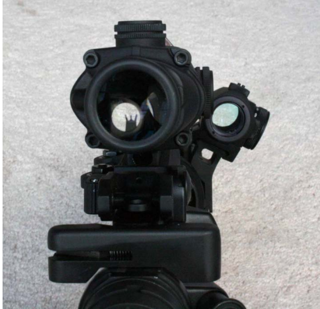
Figure 7. Soldiers view of Trijicon ACOG with Aimpoint T1 in offset mount. Source: Photograph by author.
