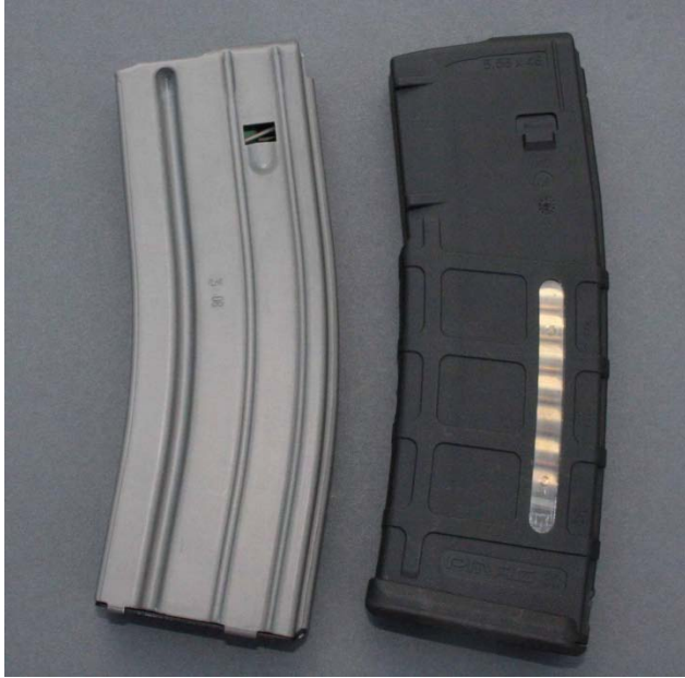
Figure 8. Comparison of standard issue magazine with Magpul PMAG with window. Source: Photograph by author.
