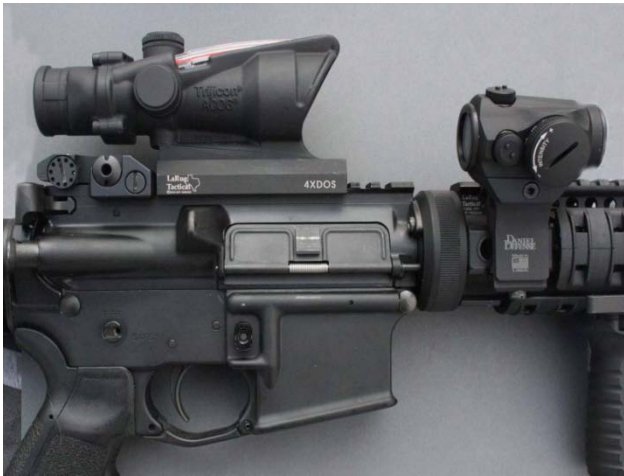
Figure 6. Trijicon ACOG with Aimpoint T1 red dot sight in offset mount. Source: Photograph by author.
