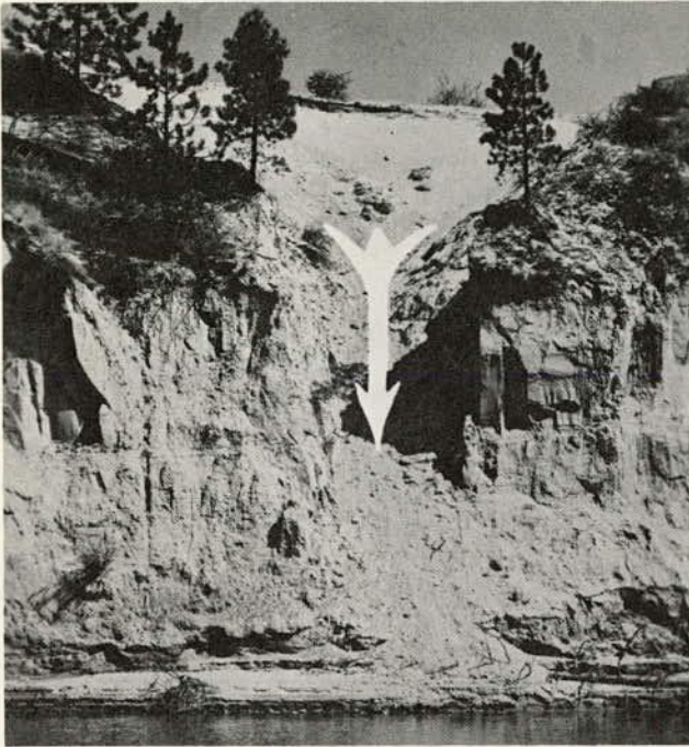
Figure 2.24. Dry sand flow in Columbia River valley (2.182). Material is sand over lake-bed silt; dry sand from upper terrace flowed like liquid through notch in more compact sand and silt below.
