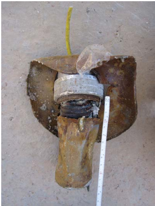
Shows the fire train from the partially exploded IED allegedly recovered at the site of the incident in Jobar, Damascus.
