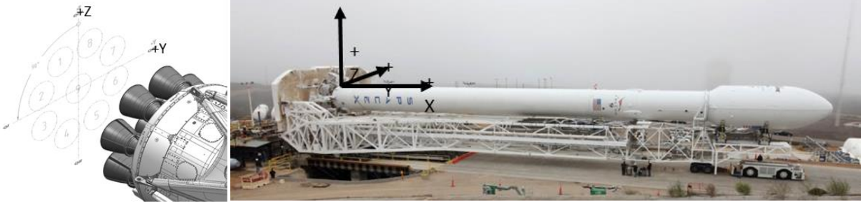
Figure 2-4: Falcon vehicle coordinate frame
