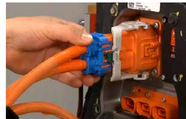
Follow the Service Information procedures to properly remove or connect a high voltage connector.
