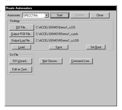
This dialog is designed to simplify creating DO files, building net classes, and specifying command line options. SPECCTRA uses a different command file format called a DO file to define the routing strategy. The **Strategy** button in this dialog is replaced with a **DO File** button.
