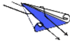
Flow with Leading Edge Vortices
