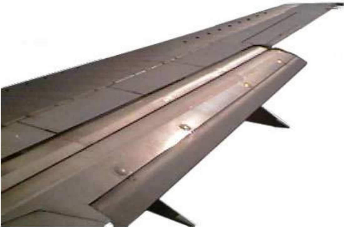
Figure 2. The triple-slotted flap system used on a 737.
