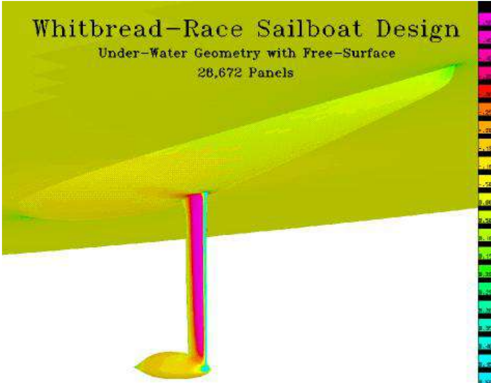
Hull, keel and bulb arrangement of Whitbread-race sailboat (courtesy of Dr. J. C. Vassberg)
