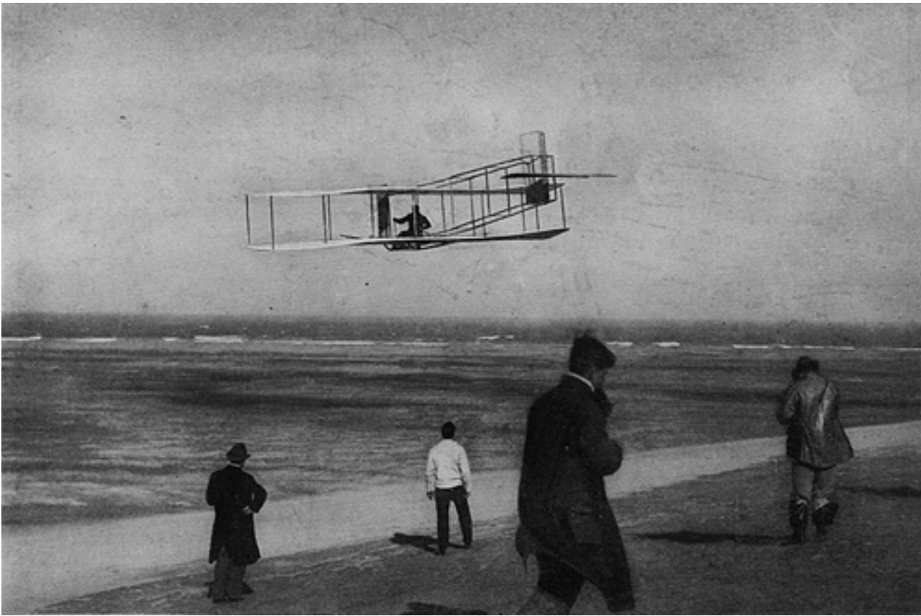
Orville Wright soars a glider in 50 mi/hr (80 km/hr) winds for 10 minutes at Kitty Hawk, Oct. 24, 1911. This was one of the first applications of a aft horizontal tail on the Wright aircraft. From Aero Club of America Bulletin, Jan. 1912.
