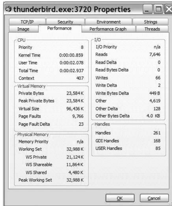
Figure 6.4 The properties window from Process Explorer reveals detailed statistics about the process in question.
