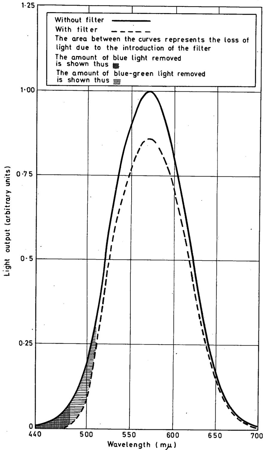
Fig.2. LIGHT OUTPUT AT DIFFERENT WAVE LENGTHS OF A SOURCE WITH A COLOUR TEMPERATURE OF 2854°K WITH AND WITHOUT A SELECTIVE YELLOW COLOUR FILTER AS DESCRIBED BY DEVAUX (1)
