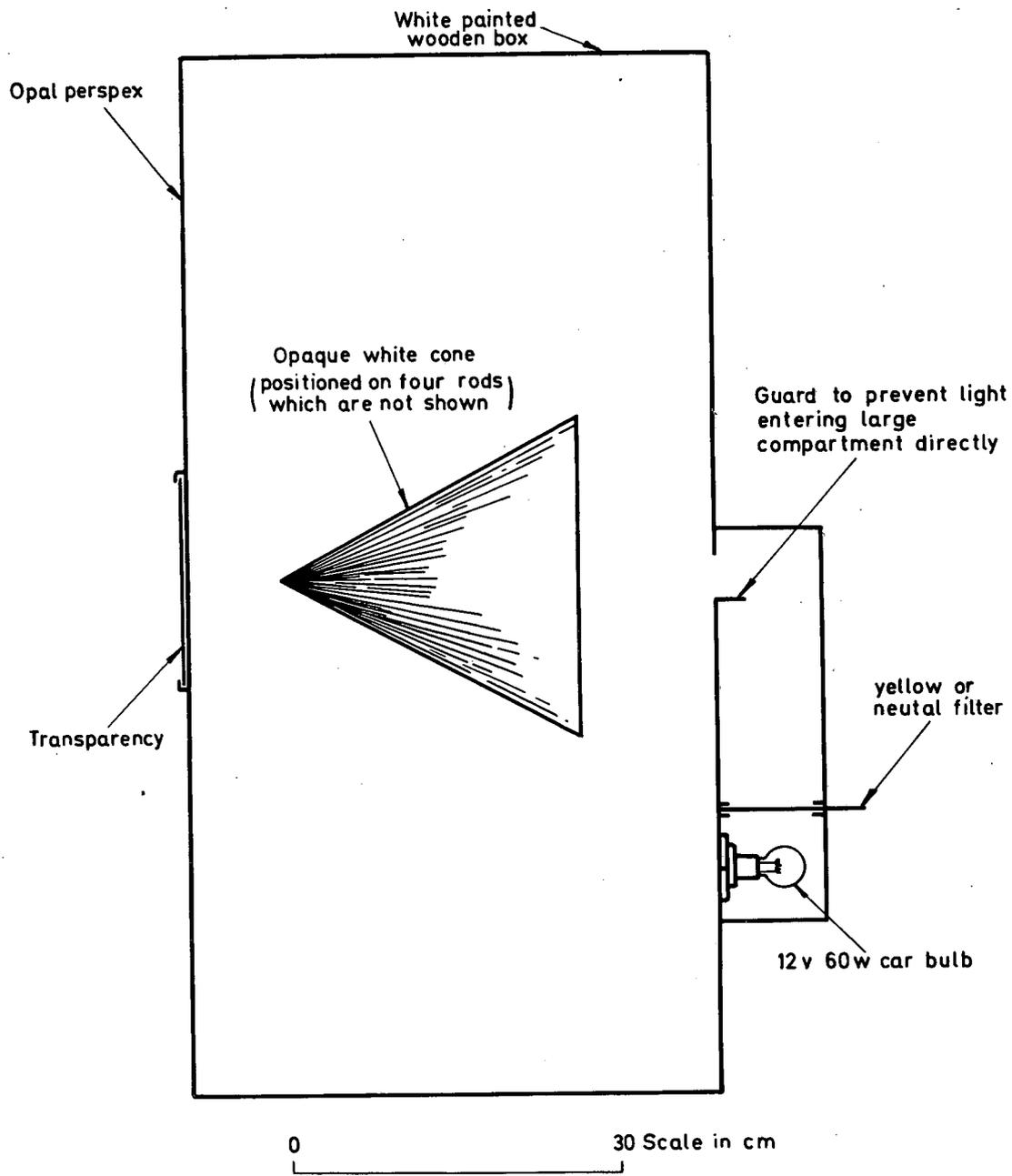
Fig. 3. SECTION THROUGH PLAN VIEW OF THE ILLUMINATING SYSTEM
