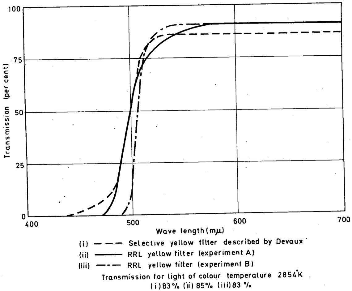
Fig.1. SPECTRAL TRANSMISSIONS OF YELLOW FILTERS USED IN FRANCE AND IN THE RRL EXPERIMENTS
