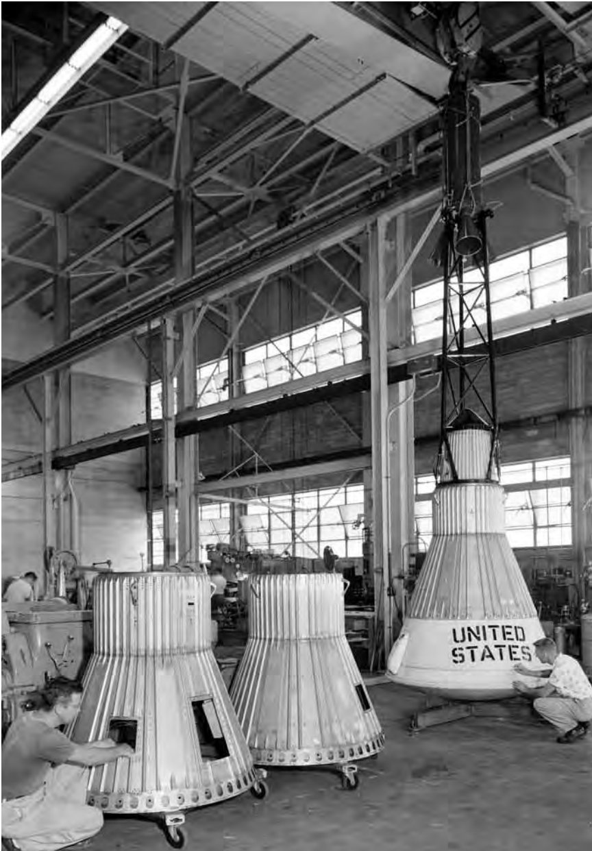
Assembling the Little Joe capsules. The capsules were manufactured “in-house” by Langley Research Center technicians. Three capsules are shown here in various stages of assembly. The escape tower and rocket motors shown on the completed capsule would be removed before shipping to Wallops Island. These test articles met the weight and center-of-gravity requirements of Mercury and withstood the same aerodynamic loads during the exit trajectory. NASA L59-4944.
