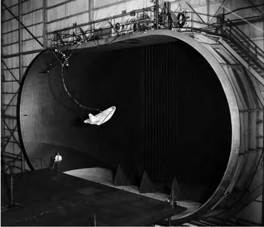
HL-10 lifting body model in NASA Langley Research Center's Full-Scale Tunnel in 1963. NASA L-1963-06125.
