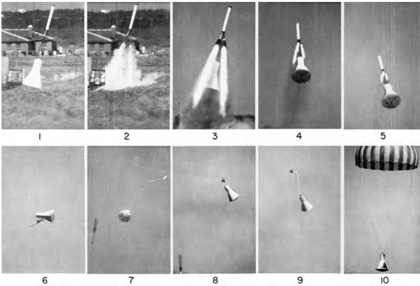
The sequence of events, from launch to parachute opening, of a beach abort test for the Mercury capsule with a launch escape motor on April 13, 1959. NASA L59-2768.
