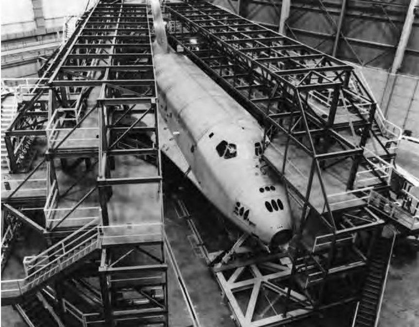
The Space Shuttle structural test article undergoing tests in the Lockheed facility in Palmdale, CA. This airframe, STA-099, was subsequently refitted for orbital flight and became the Challenger (OV-099). NASA.
