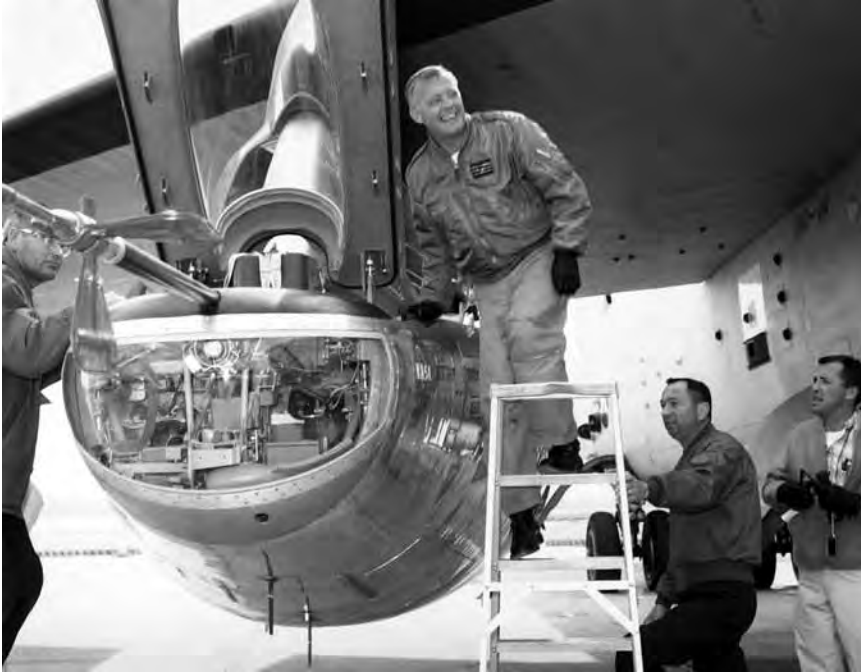
Jay L. King, Joseph D. Huxman, and Orion D. Billeter assist NASA research pilot Milton O. Thompson (on the ladder) into the cockpit of the M2-F2 lifting body at the NASA Flight Research Center. The M2-F2 is attached to the same NB-52 wing pylon used by the X-15 program. NASA EC66-1154.
