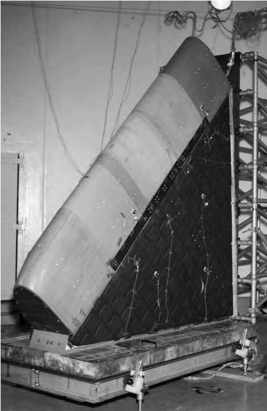
This 1979 structural test article of the Space Shuttle wing shows the reinforced carbon-carbon and tile structure. NASA.
