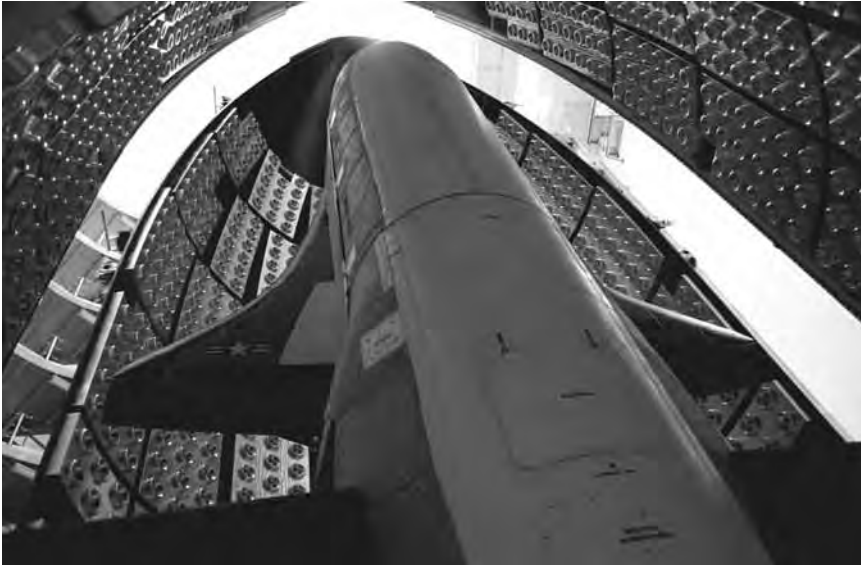
The X-37B Orbital Test Vehicle waits in the encapsulation cell at the Astrotech facility in Titusville, FL, on April 5, 2010. Half of the Atlas V 5-meter fairing is visible in the background. U.S. Air Force.
