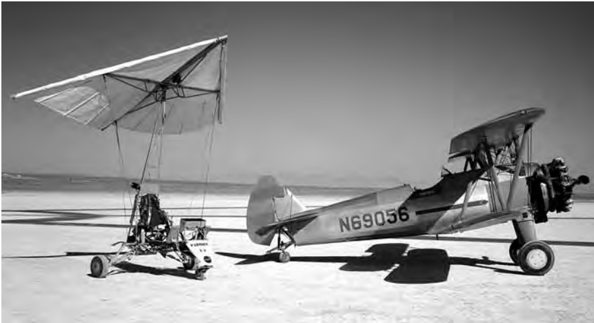
The Parasev-1-A (Paraglider Research Vehicle) and the tow airplane (450-horse power Stearman sport biplane) sitting on Rogers Dry Lake, CA. The control system in the Parasev-1-A had a conventional control stick position and was cable-operated; the main landing gear used shocks and bungees with the 150-square-foot wing membrane made of 6-ounce unsealed Dacron. NASA E-8712.
