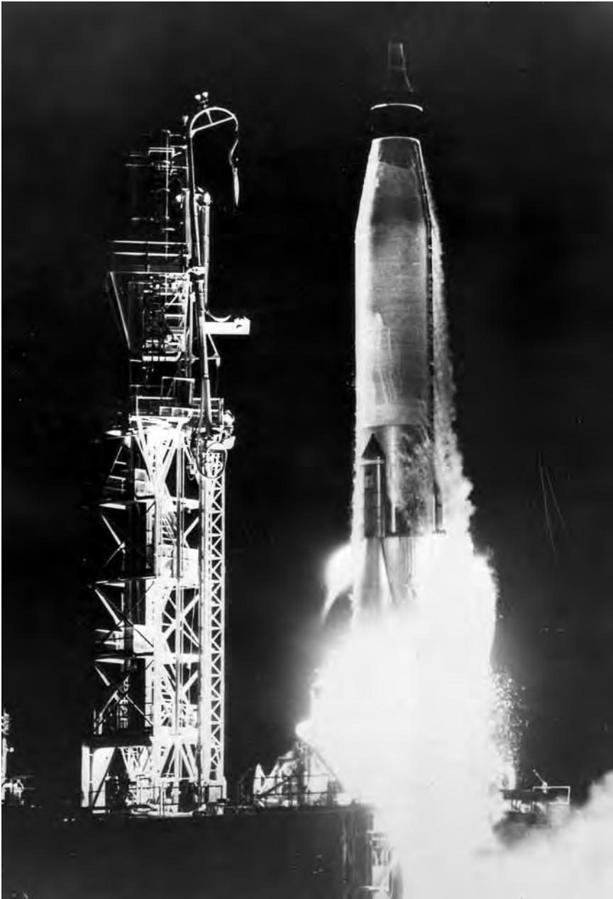
An Atlas launch vehicle carrying the Big Joe capsule leaves its launch pad on a 2,000-mile ballistic flight to an altitude of 100 miles on September 1, 1959. This boilerplate model of the orbital capsule was recovered and studied for the effect of reentry heat and other flight stresses. NASA MSFC-9139360.
