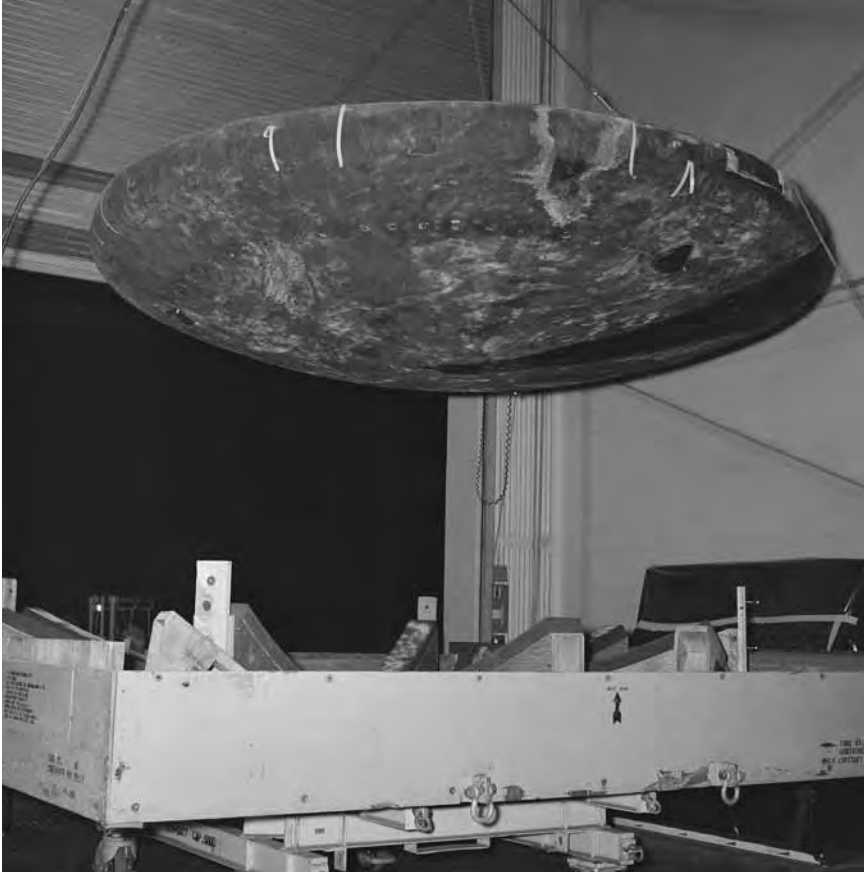
Apollo 11 Command Module heat shield inspected on November 6, 1967. NASA S67-48970.
