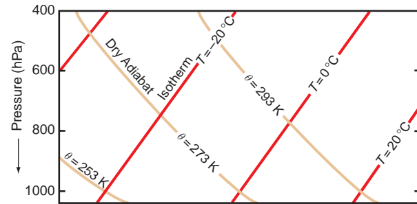
Fig. 3.7 Schematic of a portion of the skew T - \ln p chart. (An accurate reproduction of a larger portion of the chart is available on the book web site that accompanies this book, from which it can be printed and used for solving exercises.)
