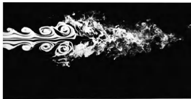
Fig. 9.3 Water tank experiments of a jet of water (white) flowing into a tank of clear, still water (black), showing the breakdown of laminar flow into turbulence. [Photograph by Robert Drubka and Hassan Nagib. From M. Van Dyke, An Album of Fluid Motion , Parabolic Press, Stanford, CA. (1982), p. 60.]
