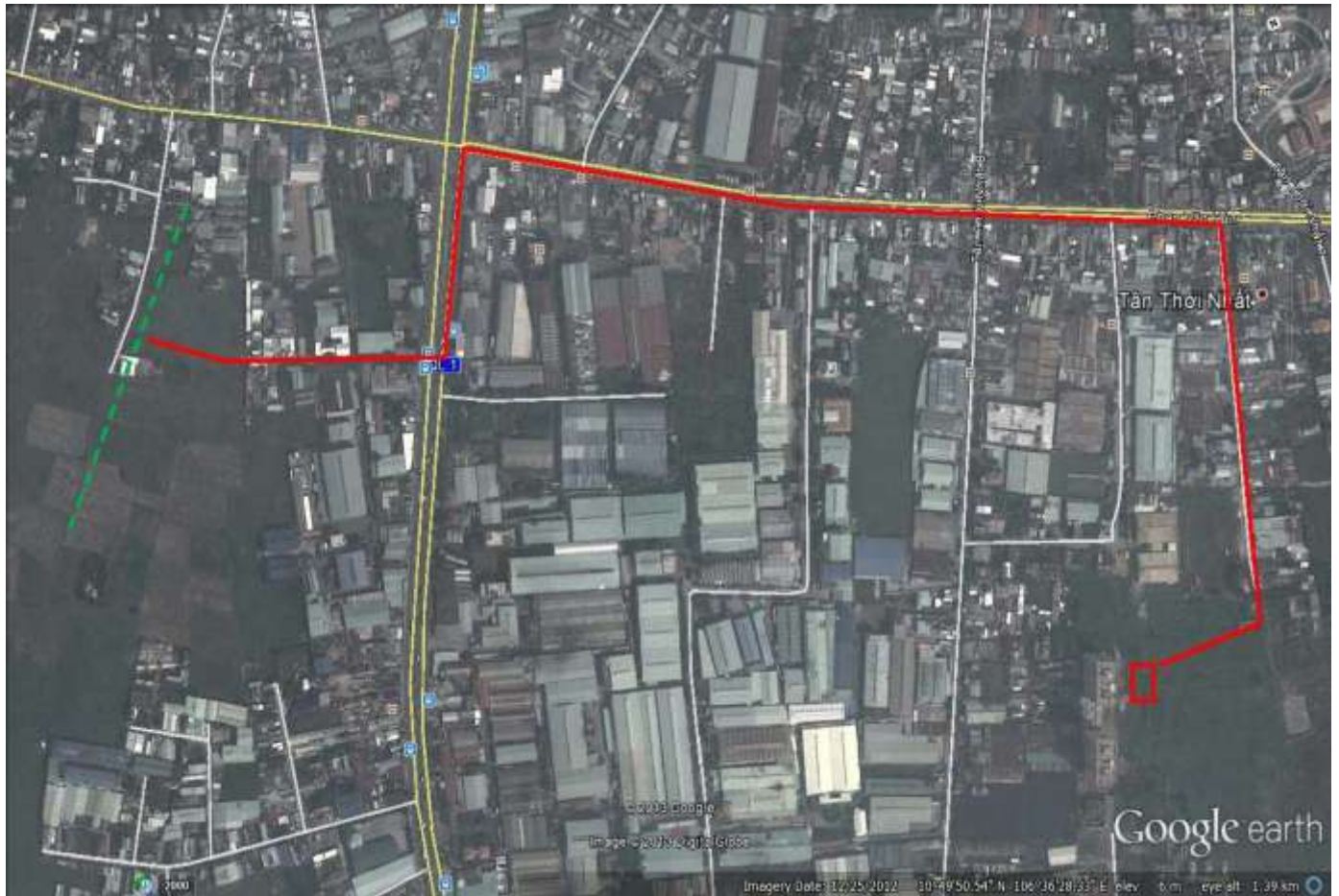
Figure 1. Route of new 110 kV UGC (red) from Hoc Mon OHL (green) to new substation
