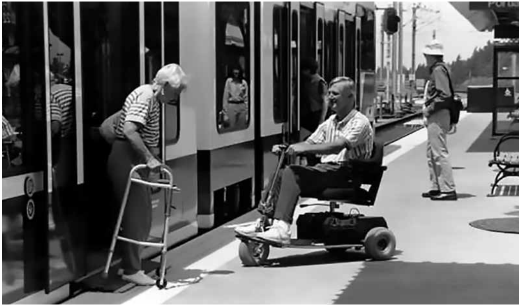
MAX type 2 low-floor vehicles, first in North America to offer roll-on boarding, 1997
