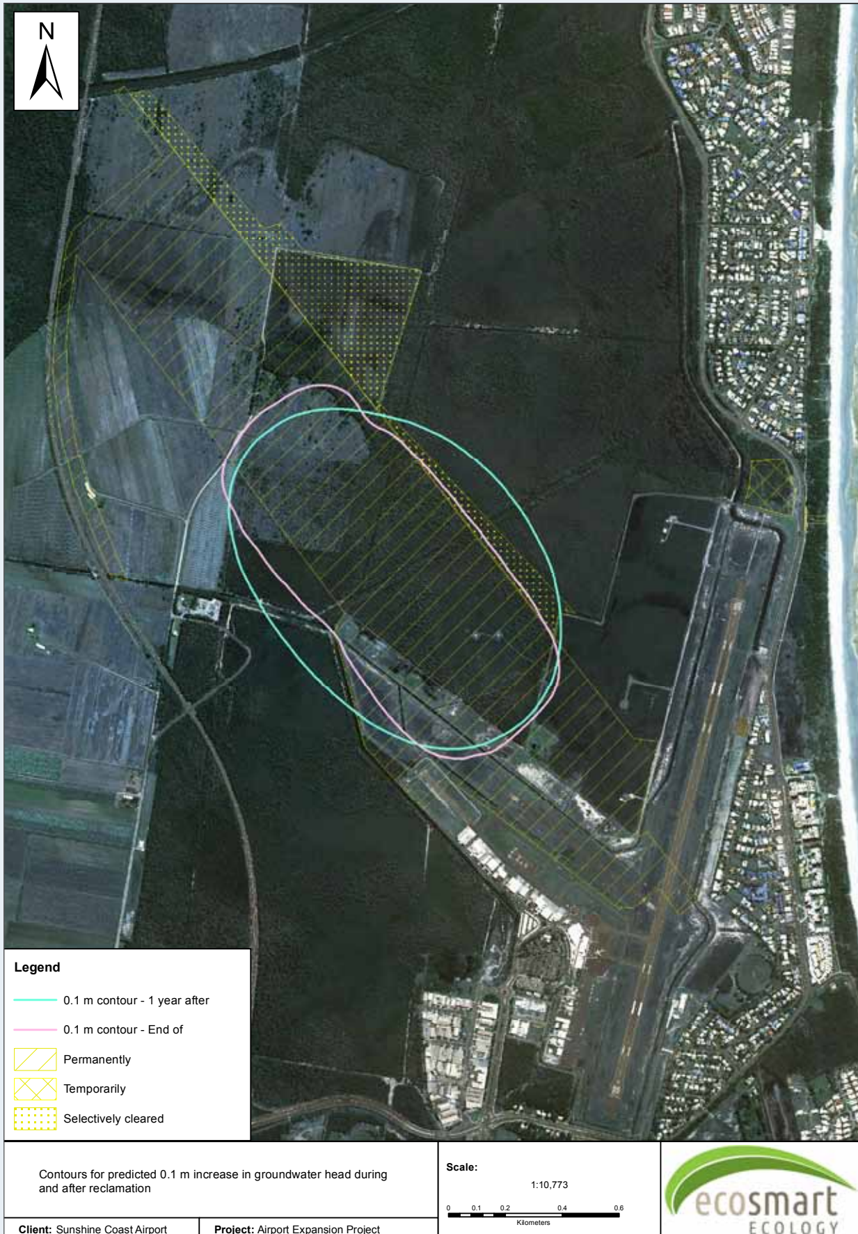
Figure 8.15c: Contours for predicted 0.1 m increase in groundwater head during and after reclamation
