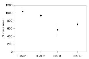
Figure 2. *Apparent surface area, four carbons.* (*Nitrogen/BET*)
