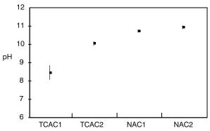
Figure 1. PZC approximation, four different carbons (Tick marks designate mean values, bars represent standard error, based on five samples
