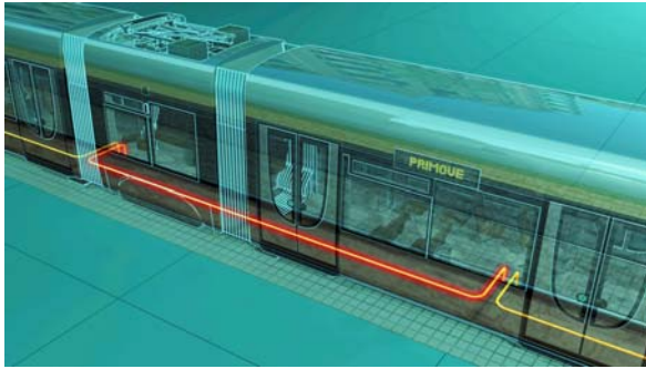
Figure 18: Underground Inductive Power (Photos courtesy of Bombardier Transportation)
