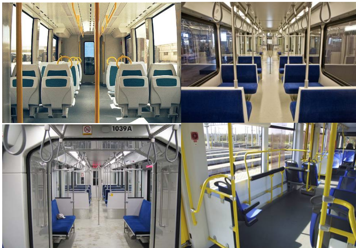
Figure 3: LRT Vehicle interior photos with areas for special needs seating
