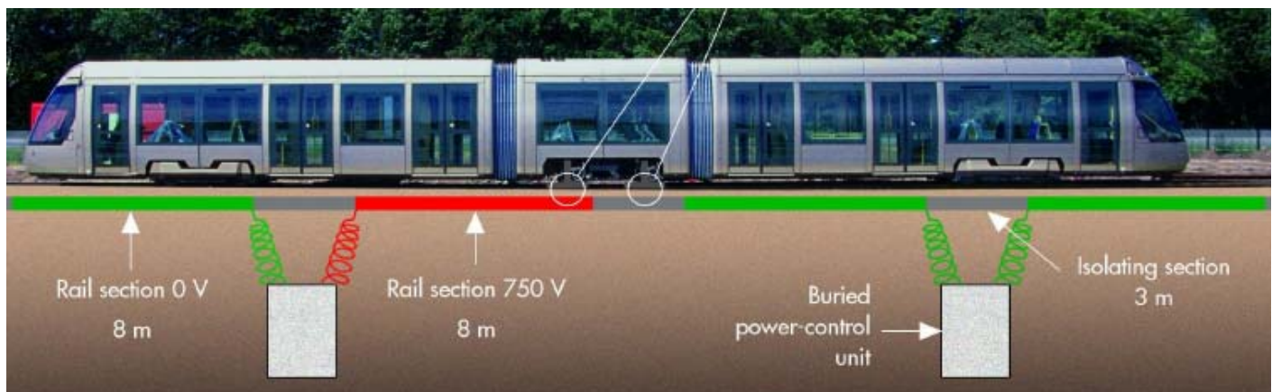
Figure 17: Alstom's APS System allows the design of a safe street level third rail system (Alstom, 2008)
