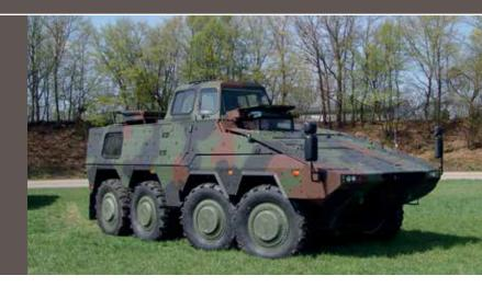
BOXER Driver Training Vehicle (DTV) provides realistic training for drivers of all BOXER variants and it permits the highest level of quality and safety of driver training. BOXER DTV consists of a standard Drive Module and the Driver Training Mission Module. Weight and ride behaviour completely match the characteristics of the Armoured Personnel Carrier.
