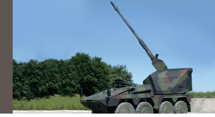
BOXER Remote Controlled Howitzer 155 mm (RCH 155) combines long range intense firepower and the fully automated Artillery Gun Module with the protection and mobility of the combat-proven wheeled armoured vehicle BOXER.
