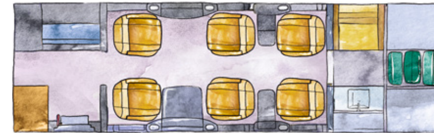
Two club seats, two single seats, one side facing seat and belted toilet (Maximum: 8 passengers)
