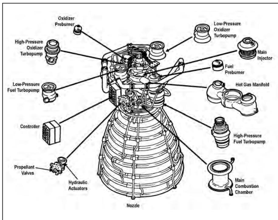
Figure 2–24. Space Shuttle Main Engine Components. (Rocketdyne)
