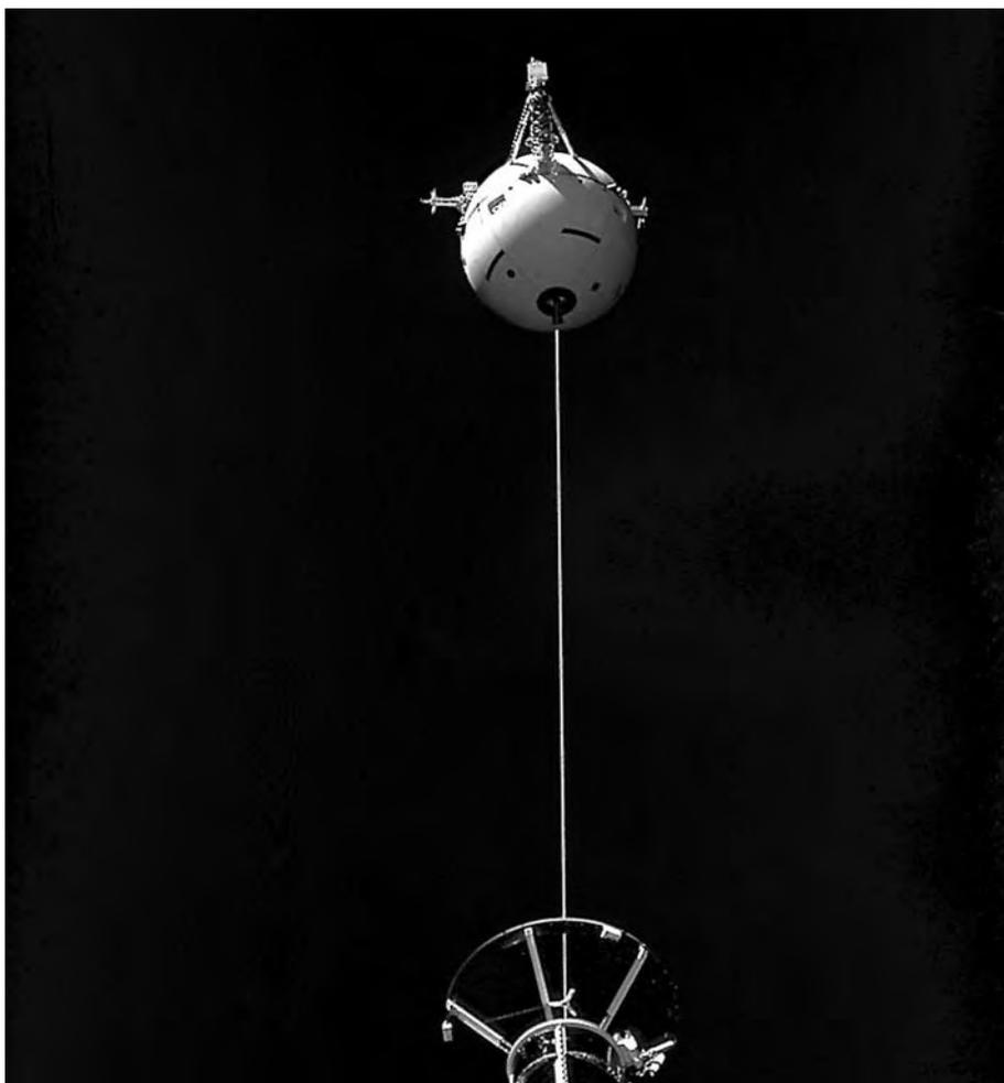
*Figure 2–28. The Magellan Spacecraft with its attached Inertial Upper Stage (IUS) Booster is in the Orbiter Atlantis Payload Bay prior to closure of the doors at T-3 days to launch. Launch of Magellan and STS-30 took place on May 4, 1989. (KSC Photo No. 89PC-0469)*
