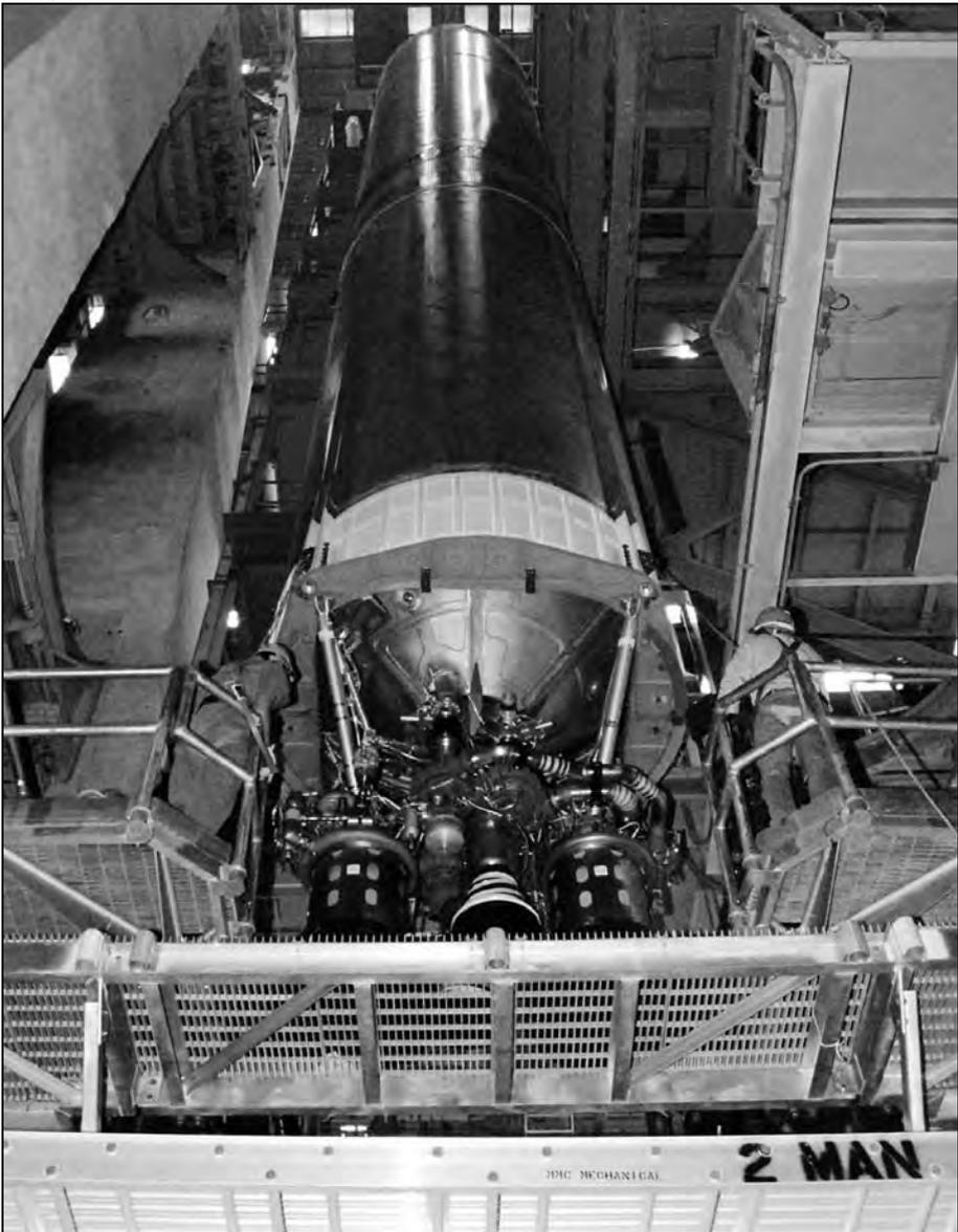
*Figure 2–21. The first stage of the Titan IV ELV that sent NASA’s Cassini Spacecraft to Saturn and its moon. Titan is lowered into a high bay in the Vertical Integration Building at Cape Canaveral Air Station to begin stacking operations, April 14, 1997.
