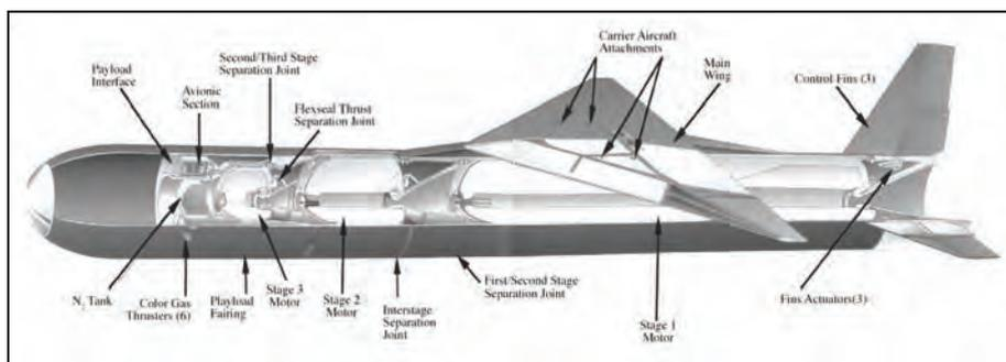
Figure 2–18. Pegasus Vehicle. (Orbital Sciences Corp.)
