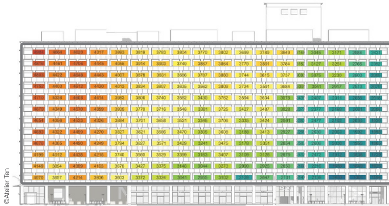
(above and right) Two façade heat studies indicate which windows will need exterior shading and which require no shading.
