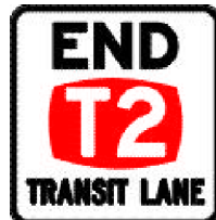
End transit lane sign (End transit lane (T2) sign) (rule 156)
