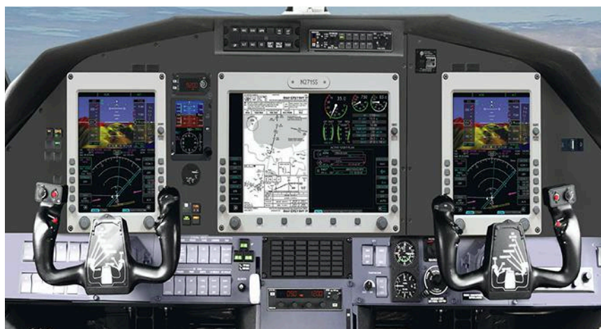
Innovative Solutions & Support FG retrofit on the Pilatus PC-12
