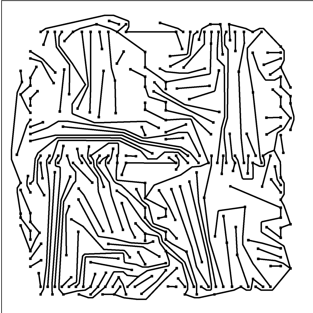
FIGURE 15 - Euclidean routing. This example shows the same layer in Figure 13 but with euclidean (any-angle) routing.
