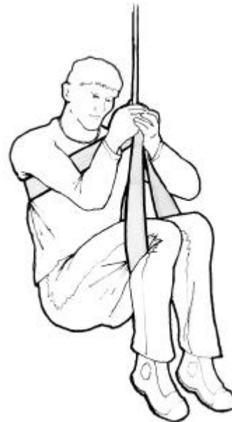
Figure 2 Suspension with a double-strop device (after Madsen) The thorax is upright and venous return is secured by elevation of the legs
