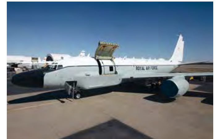
All-weather electronic surveillance aircraft based on the C-135 airframe.
