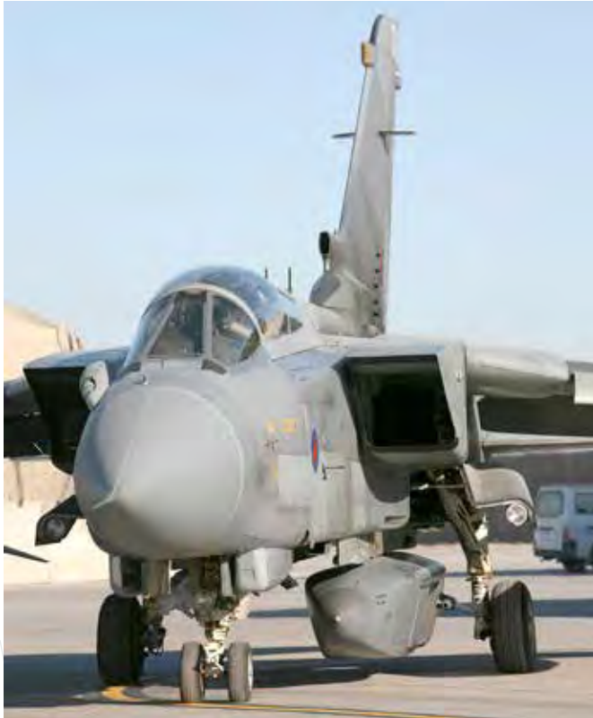
With a RAPTOR pod under its fuselage, the Tornado GR4 becomes a world-class tactical reconnaissance platform. The system continues to prove its immense utility over Afghanistan. The aircraft is shown at Kandahar Airfield. Sqn Ldr Dylan Eklund.
