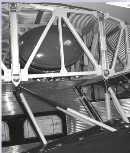
In restoration, the right side center section reveals one of three fuel tanks and motor mounting system.
