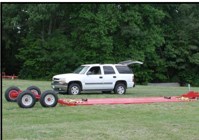
Our special trailers can lay flat on the ground if needed, so rollers can be loaded and unloaded without lifting.
