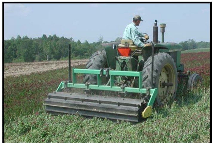
Straight-bar crimper roller: a bumpy ride at 6+ mph!
