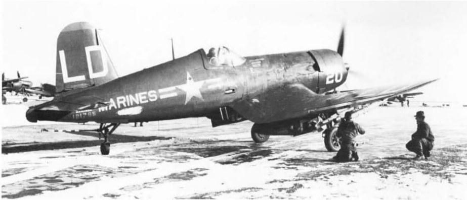
Photo by SSgt Ed Barnum, Department of Defense Photo (USMC) A130426 Marine crewmen check the loading of rockets on the rails of an F-4U Corsair flying from Yonpo Airfield early in December. Despite minimum facilities and terrible weather, the hard-working crews maintained an availability rate of 67 percent for aircraft flying from Yonpo.
