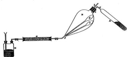
In this apparatus A is the dialkylzinc B is the receiver, containing several bulbs. C is a calcium chloride tube D is a hydrogen generator When the apparatus has been flooded by hydrogen, the tubes at b and f are sealed.
