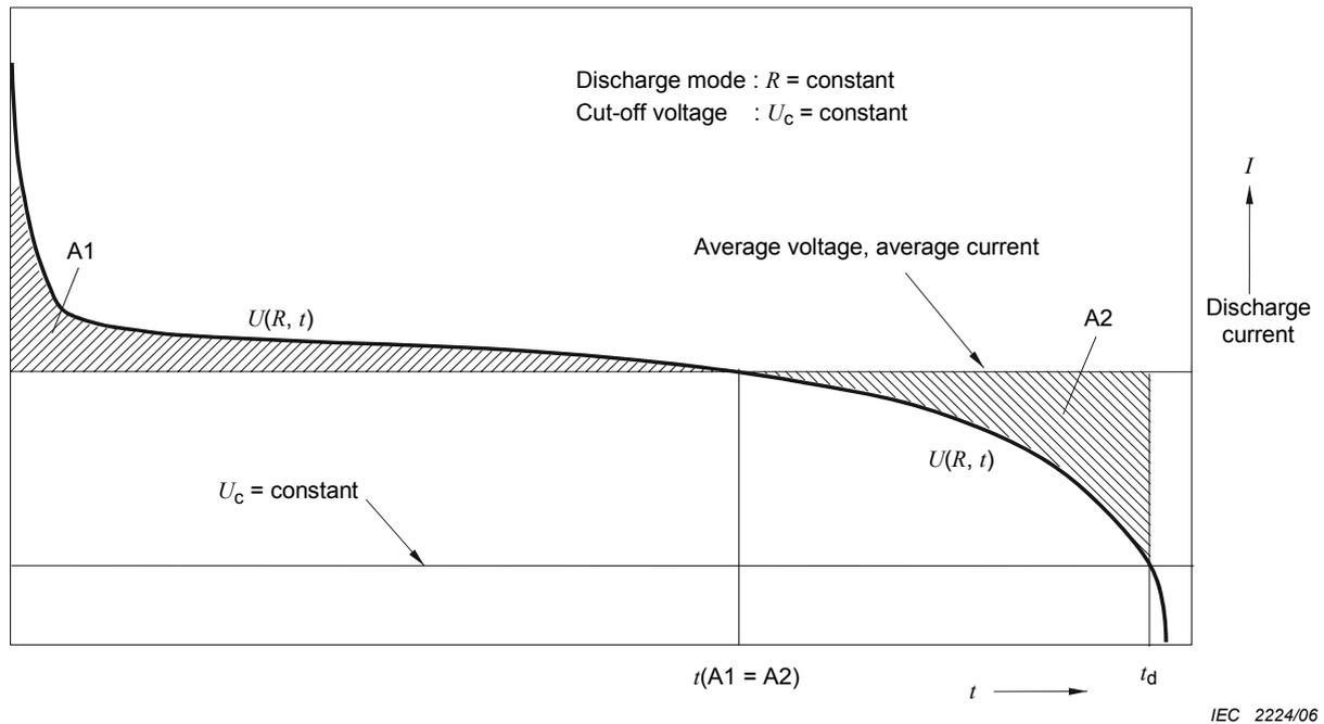
**Figure F.2 – Standard discharge voltage (schematic)**
