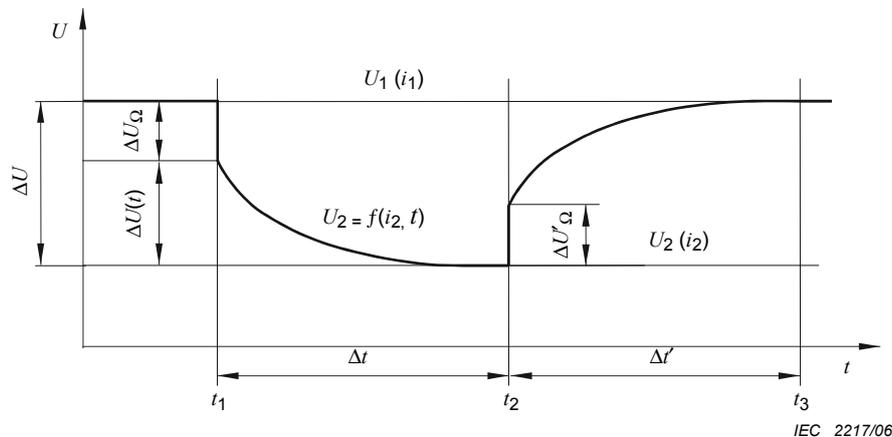
**Figure 1 – Schematic voltage transient**
