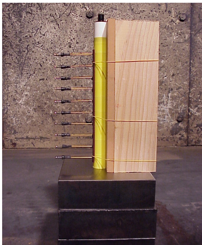
Figure 1: Velocity of detonation/detonation pressure experiment on FOX-7/EVA
