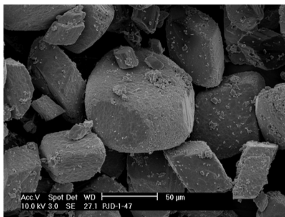
Figure 5: FOX-7 recrystallised using 45 kHz ultrasound
