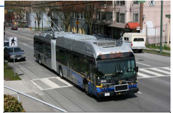
Electric trolley buses, such as this one in Vancouver, B.C., draw electricity from overhead wires.
