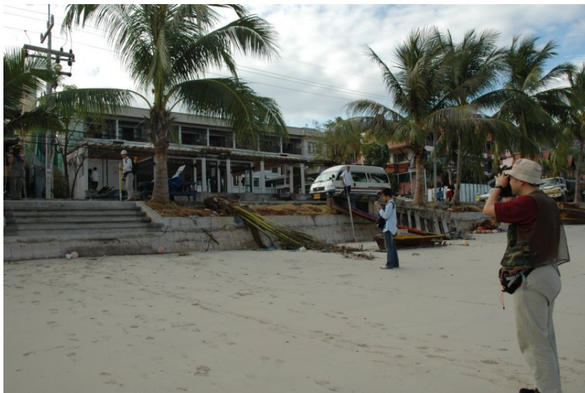
Photo 4.3 The measurement of tsunami height with the laser distancemeter
