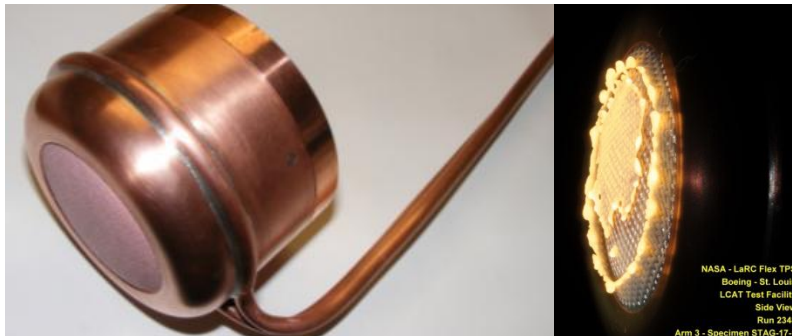
Figure 3 LCAT 3.5in Stagnation Fixture
